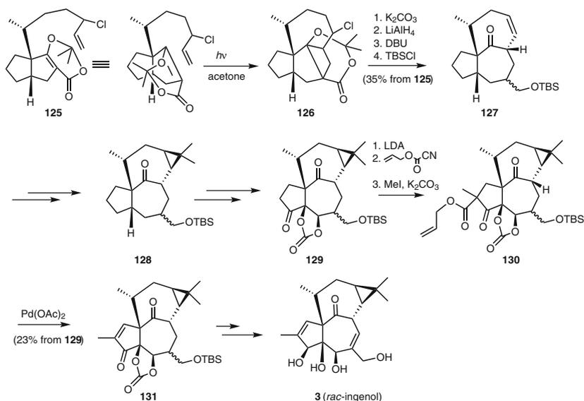
**Fig. 28** The Winkler synthesis of ingenol (DBU: diazabicycloundecene, TBSCl: *tert*-butyldimethylsilyl chloride, TBS: *tert*-butyldimethylsilyl, LDA lithium diisopropylamide)
