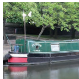
Figure 1.5 Microturbine (Rutland WG-317) charging a barge 12/24V battery (from UK manufacturer Marlec). The turbine is rated at 90W at 10m/s and 24W at 5.1m/s with a 0.9m blade diameter. (Dr Matthew Overd)
