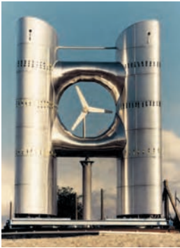
Figure 2.18 Physical testing of a prototype 2-storey building with integrated wind turbine from Project WEB (BDSP Partnership, MECAL, Xkwadmaat (NL), CRLC RAL)
