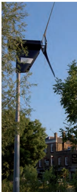
Figure 2.3 Small stand-alone turbine at the Mile End Ecology Centre, London, from UK manufacturer Proven, rated at 6kW with a 5.5m blade diameter (Ioannis Rizos)
