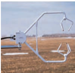
Figure 3.5 The CSAT3 sonic anemometer which can also measure turbulence (Campbell Scientific)
