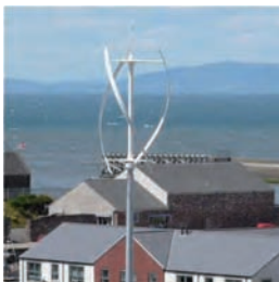
Figure 4.4 Quiet Revolution lift force type vertical axis wind turbine installed at Maryport Visitors Centre, Cumbria (Quiet Revolution)
