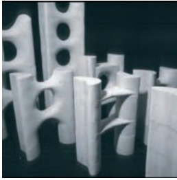
Figure 5.6 Prototype small-scale wind tunnel architectural models designed for the integration of single or multiple wind turbines (Project WEB – ibk2 University of Stuttgart)
