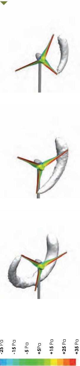
Figure 2.30 Transient 'moving mesh' CFD analysis of a small turbine, revealing pressures and lift forces on blade surfaces and modelling smoke emission from a blade tip in order to show the time dependency of these models (BDSP Partnership)
