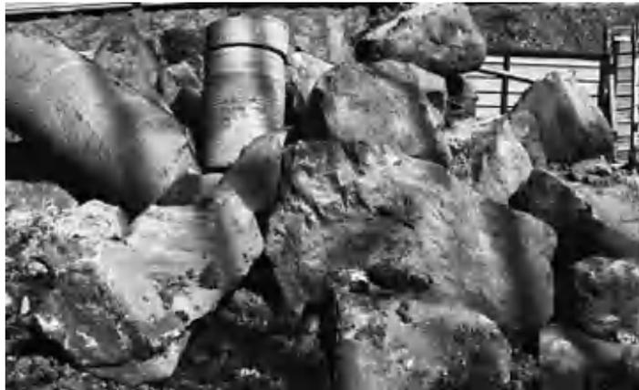
Figure B3-2.1 Angular boulders up to about 3m diameter, plus cores extracted during rock coring for large diameter piles, from a site close to Mount Sophia, Singapore.
