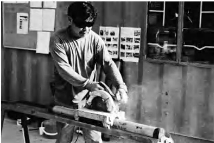
*Figure 4.29* Mazier sample plastic tube being cut for examination.
