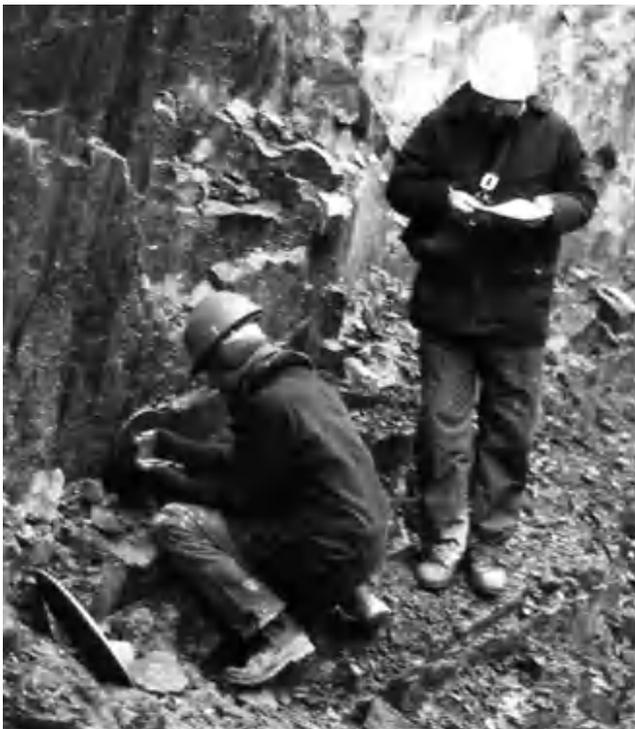
*Figure 4.17* Joint survey underway using Clar compass clinometer attached to aluminium plates. Investigation for Glensanda Super Quarry, Scotland.
