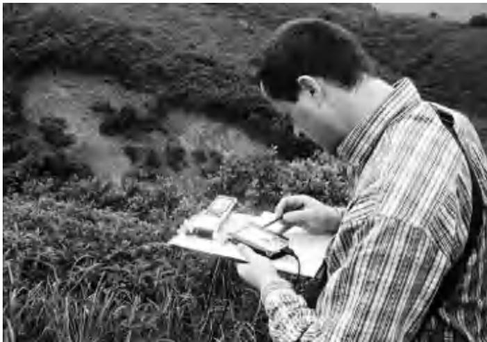
*Figure 4.9* Hand-held computer with ortho-corrected air photographs and terrain maps, used to locate and map natural terrain landslide. GPS used to get accurate locations of identified features.
