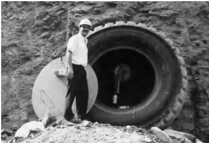
*Figure 4.43* Extensometer with claxon and flashing lights used to warn workers at Aznalcollar mine, Spain, of danger from moving slope.
