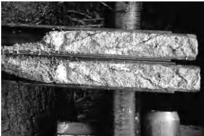
*Figure 4.32* Split spoon sample of completely weathered granite. Note presence of relict joints and lack of visible disturbance.
