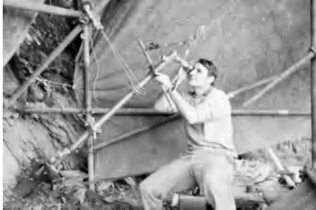
Figure B4-6.2 Borehole periscope in use.
