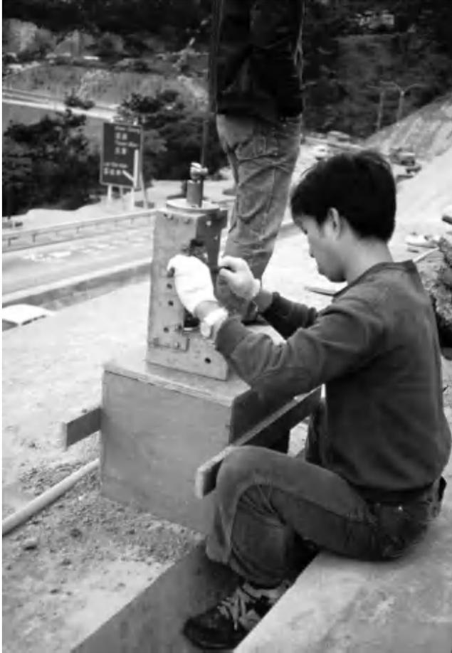
*Figure 4.11* Hand trimming a sample to size in the field, for transportation to laboratory and triaxial testing.
