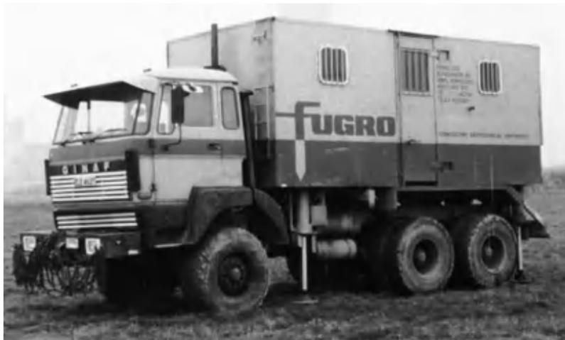
*Figure 4.35* Heavy lorry being used to conduct static cone penetrometer tests.
