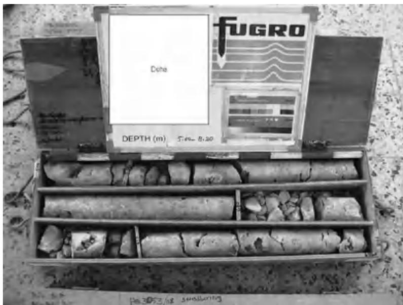
Figure B5-1.3 Example of core through Simsim Limestone (courtesy of Karim Khalaf, Fugro, Middle East).
