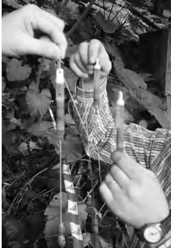
*Figure 4.41* Halcrow buckets retrieved at Yee King Road landslide investigation (Hencher *et al.*, 2008). These are unusual in that they contain sediments (from turbulent flows down the borehole). Normally, they would just contain water (or not), indicating the highest level that the water has risen in the borehole between inspections. Left side bucket is attached by fishing line to lead weights used to lower the buckets down the borehole.
