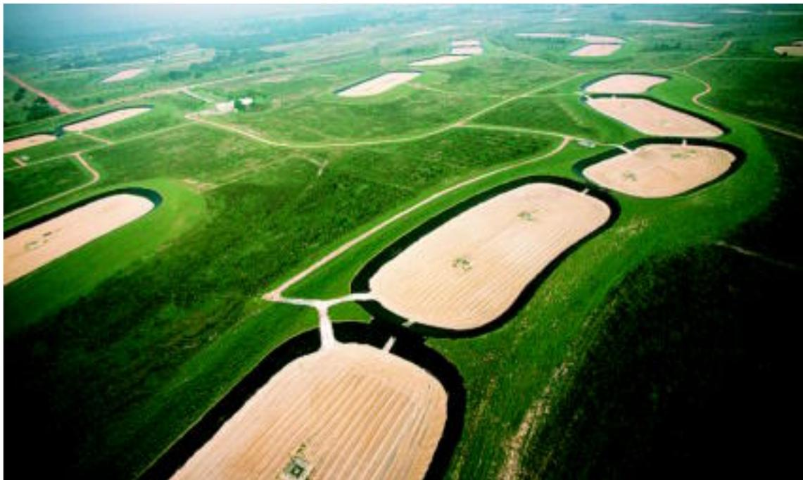
Sand and water filters working to treat and recycle sewage water for later use by citrus farmers for irrigation. © Kevin Fleming/Corbis.
