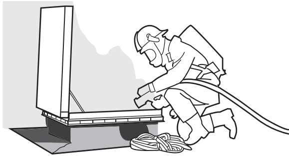
Figure 18.22 Automatic smoke ventilation hatch
