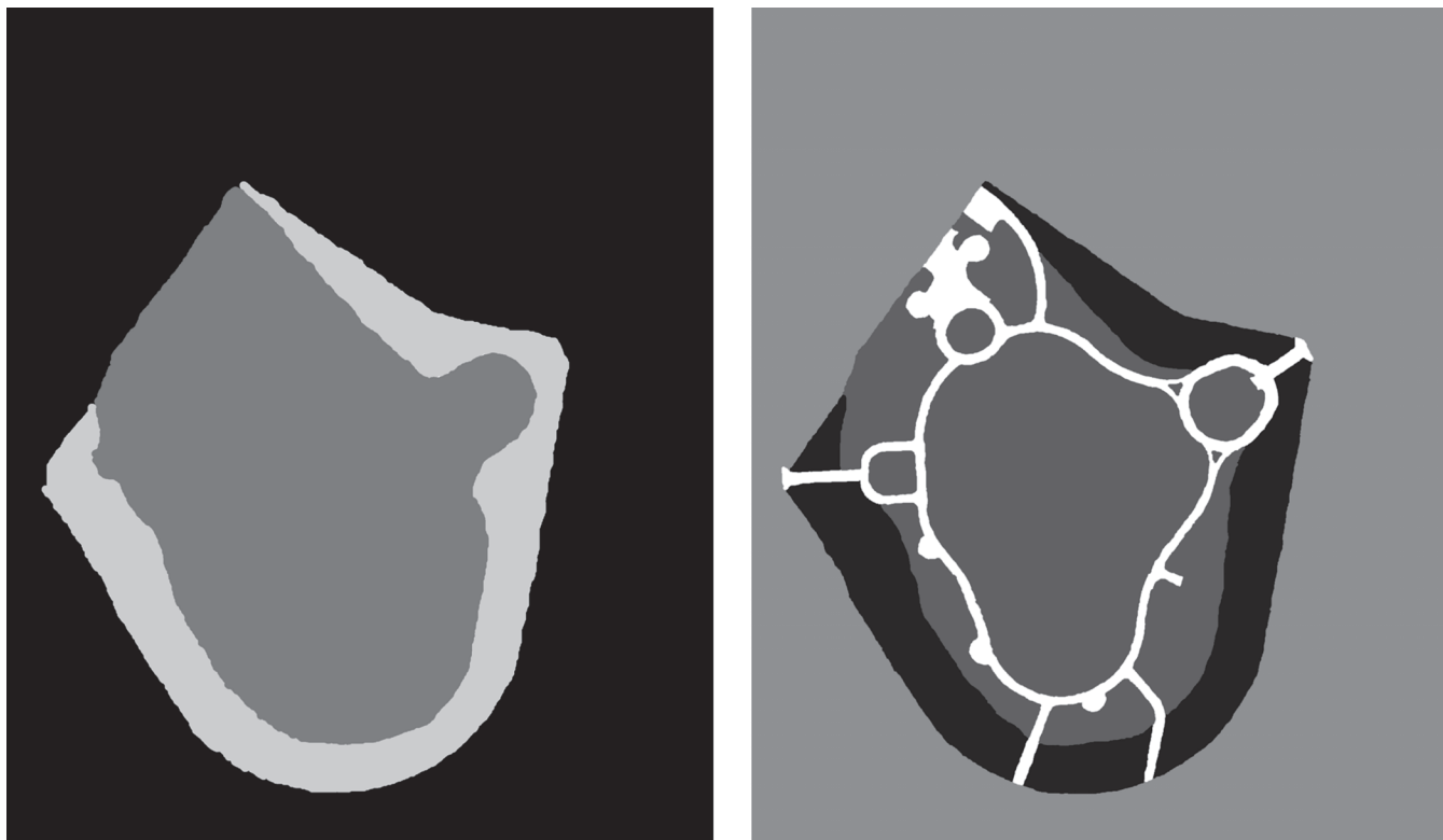
Figure 6.29. Grey scale images of Figs 2 and 3, were used to get accurate estimates of area in the various zones of each phase for RUSLE calculations.
