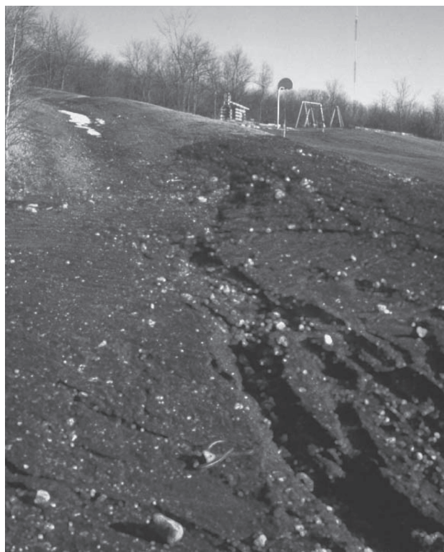
Gully erosion beginning to form where concentrated flows form after sheetflows.
