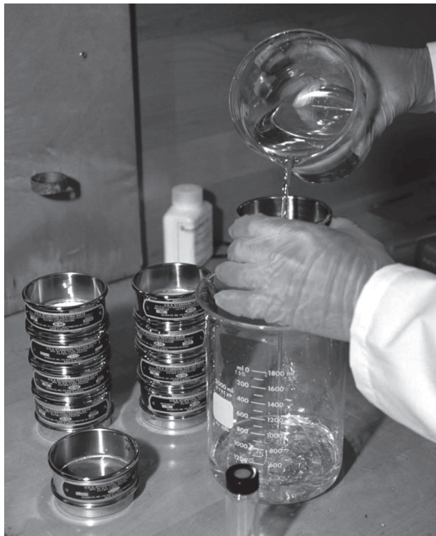
Cascading sieves (with total solids analyses after each sieve).
