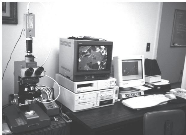
Research light microscope with automatic video analyses of particles.
