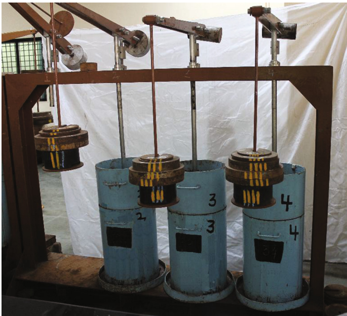
Fig. 3. Specially designed loading frame for the consolidation of clay
