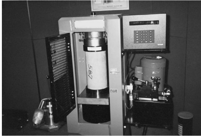
FIGURE 2.3 Testing a 6 \times 12 in cylinder in compression. (Courtesy of the Portland Cement Association.)
