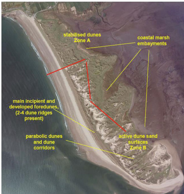
Fig. 9.7 Inch Spit dune-barrier morphometric type areas and environmental zonation (Science Direct 2013) (Photograph Source: Office of Public Works and Ordnance Survey of Ireland 2012)
