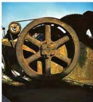
This flywheel, which operates a metal cutter, has a large moment of inertia about its center. Once it begins rotating it is difficult to stop it and therefore a uniform motion can be effectively transferred to the cutting blade.
