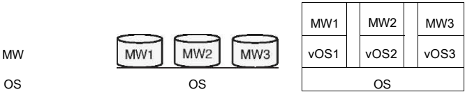
Figure 7.4 Multi-tenancy for MW layer in application tier
