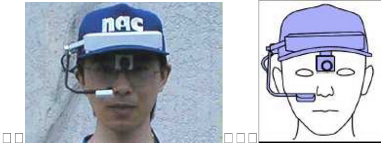
Fig. 4. Picture of Eye Mark Recorder 8 (EMR8). EMR records eye movement of subject. The recorder is lighter and does not constrain the subject's movement.
