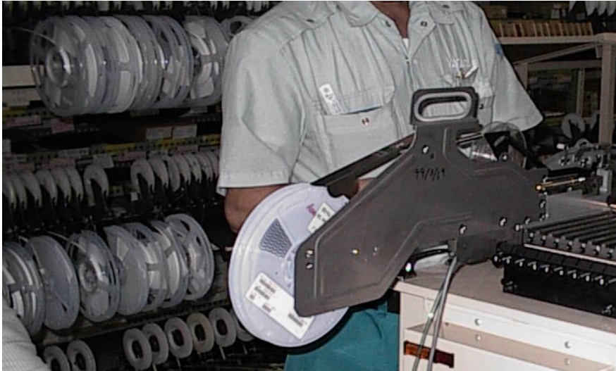
Fig. 1. One of the external change-over activities: Fixing parts to feeding mechanisms
