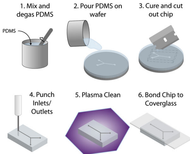
Fig. 3 Soft lithography: (1) Curing agent and polymer are mixed in a 1:9 ratio and degassed. (2) Uncured PDMS is poured over the master mold. (3) Once the PDMS has cured, the chip is cut out (4) and shaped into a chip and the inlet and outlet ports are punched. (5) Plasma cleaning exposes silanol groups on the PDMS allowing it to (6) covalently bond to a glass coverslip forming the completed microfluidic chip
