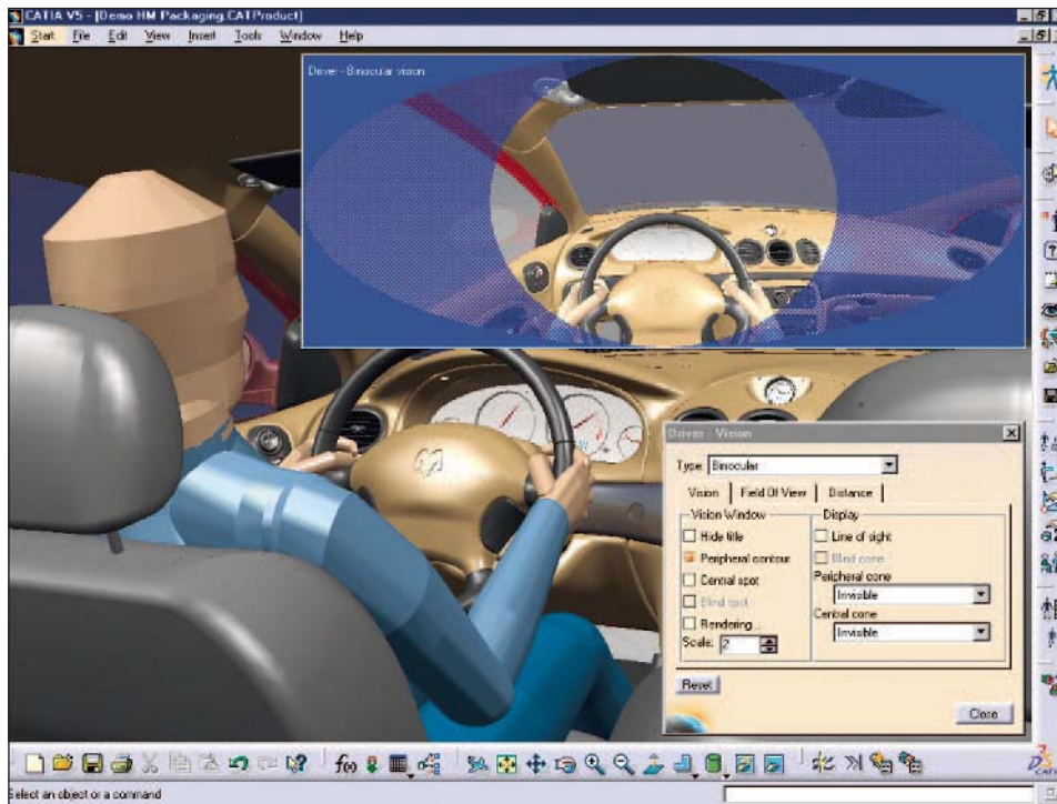
Figure 4.58 Human interaction and ergonomic simulation within a 3-D car
