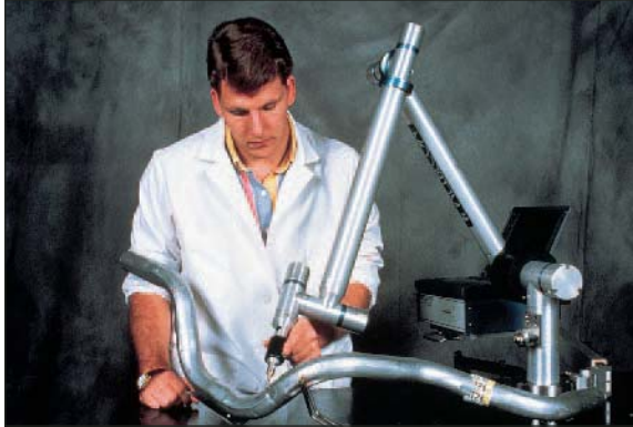
Figure 11.59 Coordinate measuring machine (CMM) used to accurately measure a part for reverse engineering or quality control
