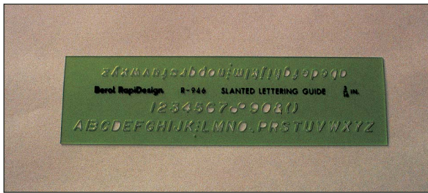
Figure 2.34 A mechanical lettering template used to assist in the drawing of text on engineering drawings
