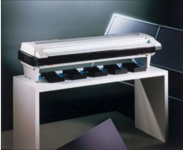
Figure 10.58 A diazo machine used to make blueprint prints
