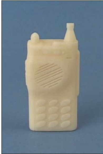
Figure 11.25 Real model of a portable hand-held radio created with a rapid prototyping system
