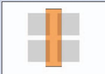
A series of overlapping boxes indicates a subtle connection between two elements: circulation (orange) and classroom units (gray). This diagram describes how these units can overlap into the hallway as instructional areas.
