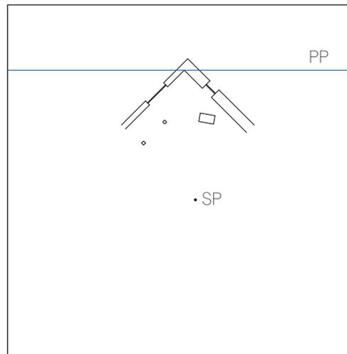
**2** Next, establish the location of the picture plane (PP). For ease of construction, this horizontal line should intersect a point on the plan, preferably a corner of the plan and one that will be seen in the perspective image.
