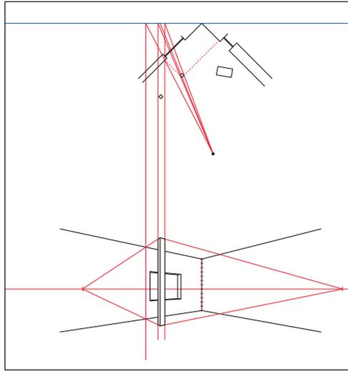
**11** Go back and forth between getting vertical information from the plan, measurements from the ML and surfaces that vanish to one of the VPs. Heights can only be taken along assisting planes for elements not along the ML. See "assisting planes," page 93.
