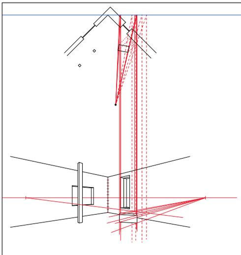
**13** All vertical measurements must be translated along surfaces if they do not connect directly to the ML (such as the chest in this drawing). That is, an object detached from a wall touching the ML must have its vertical measurements transferred across a series of perpendicular planes (even if those planes do not exist as actual surfaces in the design).
