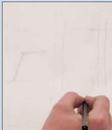
**1** Use a 4H lead to create a series of construction lines to establish the boundaries of the chair. Determine the chair's width proportion to its overall height. Continue to establish these proportions for all of the required orthographic projections. Complete this step before adding detail and line weights.
