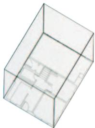
**1** Rotate your plan to an angle that highlights components of the design. Begin construction by extruding the corners of the box, using a 4H lead. Measure heights using the same scale as the plan.
