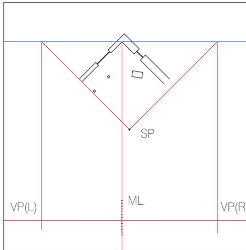
**7** Where the vertical lines from the PP cross the horizon line, you will establish the vanishing points. Call them VP(R) and VP(L). The ML should also cross the horizon line. This intersection establishes the location of the eye level for the person standing at the SP. If the person is standing on the ground, the horizon line would be 5 ft (1.52 m).
