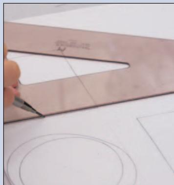
**2** Make sure to lift your triangle after making vertical lines to avoid smudging the drawing.
