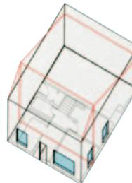
**3** Find elements that are not parallel to the plan, such as the roof, using heights taken from the corresponding elevations. Plot the height of the low and high points of the roof and connect them with a straight line.
