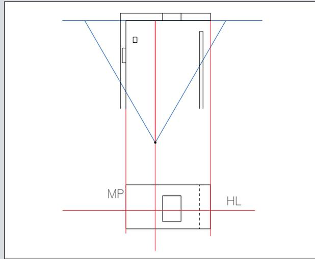
**4** Construct the back wall elevation that corresponds to the location of the PP at the same scale as the plan. Draw this in the open space below the plan. This will serve as your ML, or in this case your measuring plane (MP).
