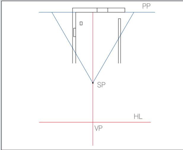
**3** Locate your HL and VP on the elevation. The VP should correspond to the appropriate height of a viewer's eyes looking into the space and can be located directly in line with your SP. The SP and VP vertically align since this is a single-view perspective with one focus.
