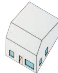
**4** Darken in those components of the construction lines that are visible as elevation lines in HB lead. You can leave the lightly drawn construction lines on the drawing.
