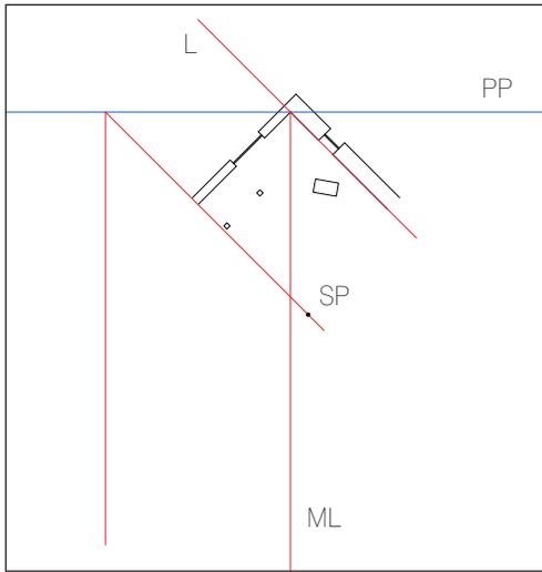
**4** To determine the location of the vanishing points it is important to follow these instructions exactly. From the SP, and using your adjustable triangle, draw a construction line parallel to line L of the plan that intersects the SP and crosses through the PP. Repeat on the other side for R.
