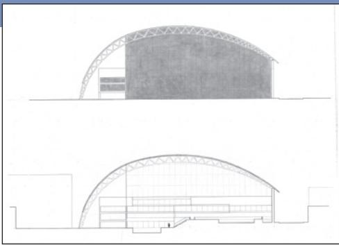
This drawing combines a building elevation and section, making the relationship between the two clear.
