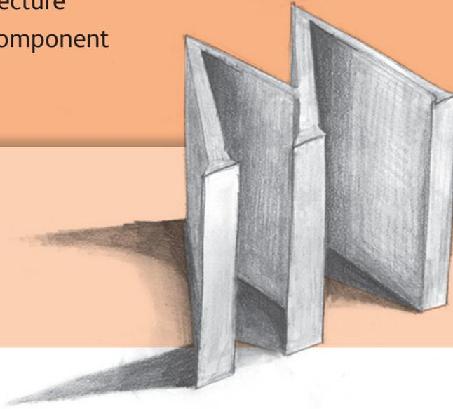
Shade and shadow added onto orthographic drawings gives a three-dimensional characteristic to a drawing by emphasizing the depth and space through light and how it interacts with surfaces. Shadows expose the physical relationship between the elements in the space that are receiving the light and the elements that are creating the shadow, the wall, window cutout, and so forth.
