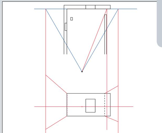
**6** Vertical lines are obtained through the same method as the 2-point perspective (see page 90). Method: SP to the point on the plan; where the line crosses the PP drop a vertical line down.
