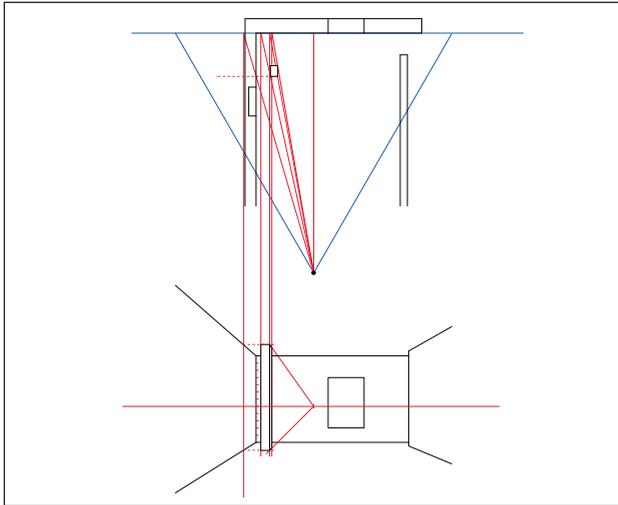
**7** Continue depicting vertical data through the previously described method (see page 95). Use the assisting planes to find the heights of the elements not connected to the ML/MP.
