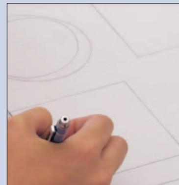
**3** As you develop the composition, make sure that the line weights in one elevation match the line weights for all the elevations on the same page. Consistency is important.
