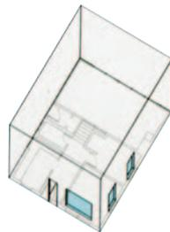
**2** Continue using construction lines, but start to add detail like doors and windows. Take vertical measurements to determine the height of the window off the ground.
