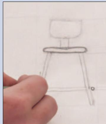
**2** Use an H lead to begin to darken the elements that are seen in elevation. The construction lines remain the lightest line weight on the page and should, at this point, begin to fade naturally as other, darker, lines appear to become more dominant.
