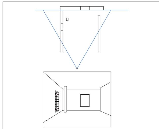
**10** The finished perspective. The CV sets the parameters of the box.
