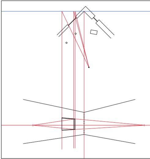
**10** Draw a second construction line, starting at A (the intersection of the first construction line and the PP) perpendicular to the PP into the perspective image area. Repeat for all lines in a given element. Cross the vertical lines with height lines obtained from the ML.
