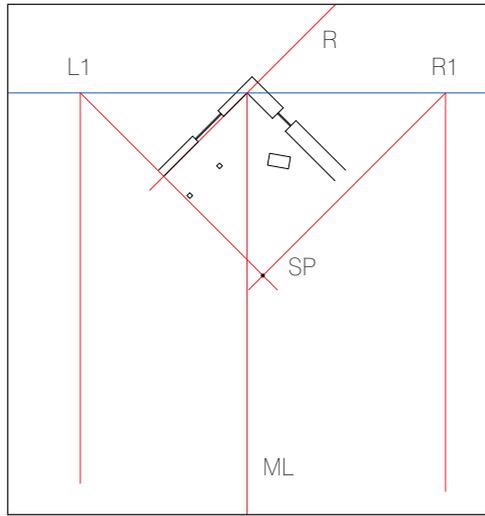
**5** Label the intersections of lines L and R with the PP L1 and R1. At R1, the intersection of the construction line and the PP, draw a vertical construction line, perpendicular to the PP into the open space of the page. Repeat at L1.
