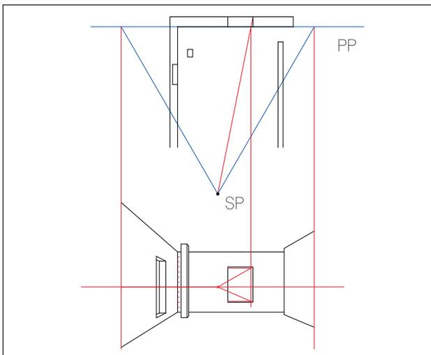
**9** Show the depth of the wall at the window opening. Extend a line from the SP through a point on the plan to where it crosses the PP and drop a vertical line down. Use measurements from the MP to draw the corners receding to the VP.
