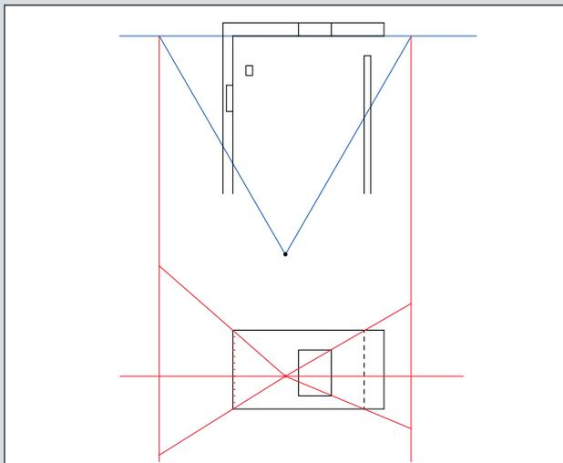
**5** Start the drawing by connecting the VP to each of the four corners of the elevation. Extend these lines beyond the limits of the elevation. This will provide the parameters of the room: walls, floor, and ceiling.
