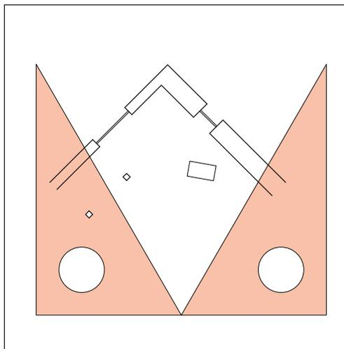
**1** Use two 30/60/90 degree triangles to establish the cone of vision. The point of the two triangles indicates the location of the SP. Tape down the plan and lay a large piece of trace or vellum overtop. Place the sheet of paper so that it covers the entire plan and leaves room at the bottom for the image.
