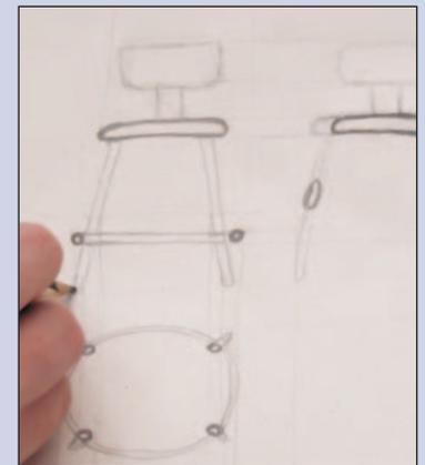
**3** Use an HB lead to begin to darken in the elements that are cut in section. Section cuts are continuous and shall not be left open-ended. Make crisp dark lines with a sharp lead. The light construction lines should remain on the drawing.
