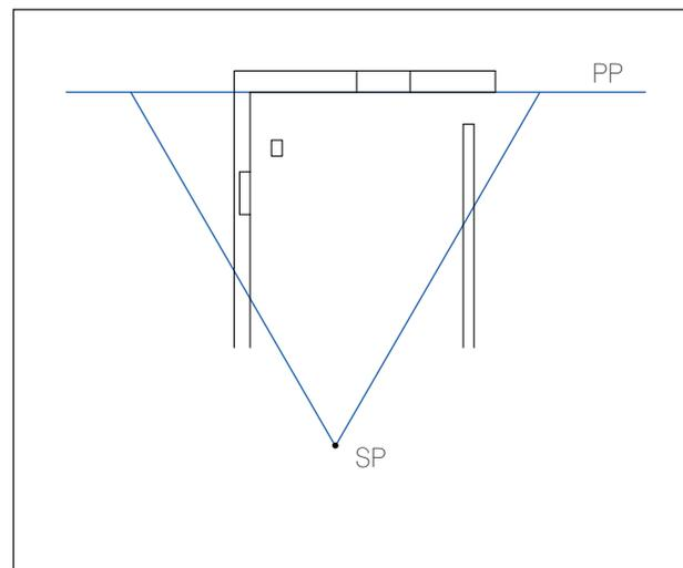
**2** Draw the PP to coincide with the back elevation for ease of construction. That is, the horizontal line demarcating the PP should cross the front edge of the wall. Blue lines indicate the cone of vision (CV).
