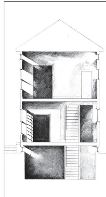
By including a profile of a person in the section you can instantly understand the scale of the space. The figure is never drawn in section, but is rendered abstractly.
