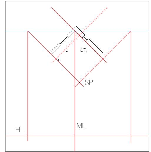
**6** At this point, you can establish the horizon line (HL) for the drawing. The horizon line can be placed anywhere on the paper and will establish the location of the perspective image. In this case, locate the HL between the plan and the bottom of the page. This should allow you enough room to construct the perspective image. The horizon line is a horizontal line, parallel to the PP.
