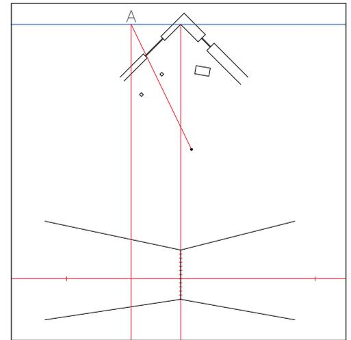
**9** To obtain vertical information, you must follow a two-step process. Draw a construction line that intersects the SP and any point on the plan and continue it through the PP (label A at the PP).
