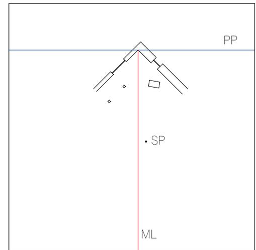
**3** Draw a vertical line from the intersection of the PP and the plan to establish the measuring line (ML). This line should extend into the white space left open for the image construction.
