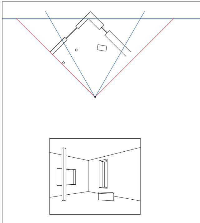
**14** Finished perspective. The CV (shown here in blue) establishes the box around the perspective.
