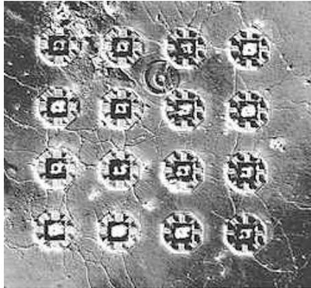
**Figure 12.12.** The neurochip, under development at the Pine Lab and Micromachining Laboratory, California Institute of Technology, allows microelectronic interfacing with individual neurons in a biological neural network [130] (image by courtesy of Pine Lab, Caltech). Reproduced from Maher *et al* [130], © Elsevier 1999.
