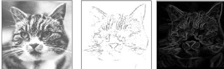
**Figure 2.7.** Input (left) to and result (right) from the Sobel gradient operator.
