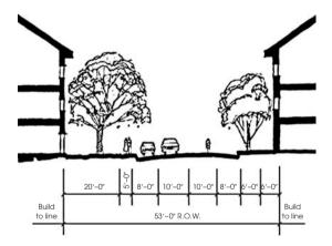
**Figure 4.9** Typical 'Street Section' Drawing. Properly proportioned sections – vertical slices through buildings and spaces – effectively engage the three-dimensional qualities of a design proposal by illustrating the heights and relative sizes of buildings, trees, people and cars.
