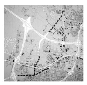
**Figure 8.4** Main Road Extensions Plan. This drawing illustrates the new highway planned by the city and state to improve north–south connectivity. We suggested substantial design revisions to turn this road into a pedestrian-friendly boulevard to serve adjacent neighborhoods as well as moving traffic from other parts of the city.
