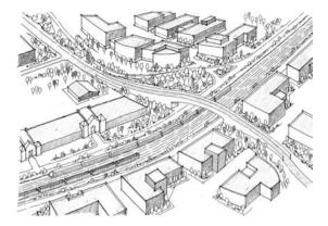
**Figure 8.3** Axonometric View of the New Road Bridge at the Fairgrounds Station. This three-dimensional sketch was crucial in obtaining agreement between the city highway engineers and the university administrators regarding new road construction to relieve congestion at this busy intersection.
