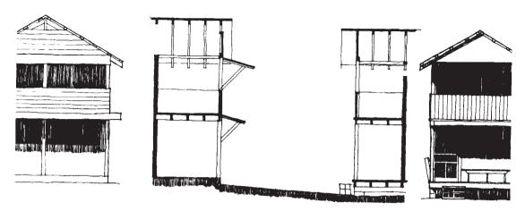
**Figure 4.1** Section Through a Typical 'Street' at Neshoba County Fair. This drawing illustrates how porches and verandas on the building façades facing the public space of the 'street' may vary in detail and size but not in their basic form and orientation. The requirement for all structures to include these spaces in their design contributes hugely to the exciting interplay of public and private spaces throughout the Fair. See also Plate 2. (*Drawing courtesy of Robert Craycroft*)
