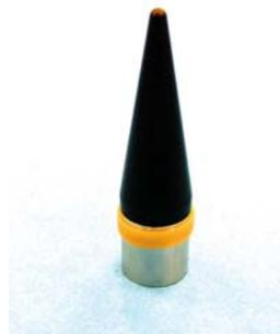
**Fig. 7.10a.** Mount a fixing rubber on a mounting tool
