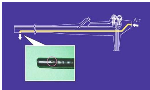
**Fig. 2.3.** Comparison of EN-450P5 and EN-450T5 **Fig. 2.4.** Air route built into the scope
