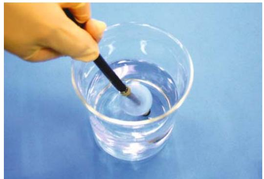
**Fig. 7.13.** Check the endoscope balloon for air leaks
