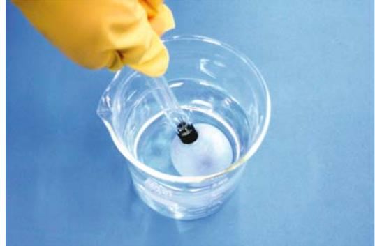
**Fig. 7.5.** Check the overtube balloon for air leaks
