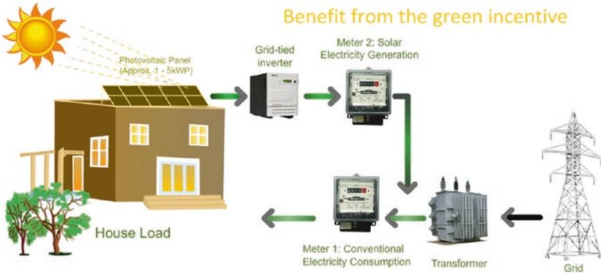
Fig. 11 Graphical representation of rooftop solar PV system [29]
