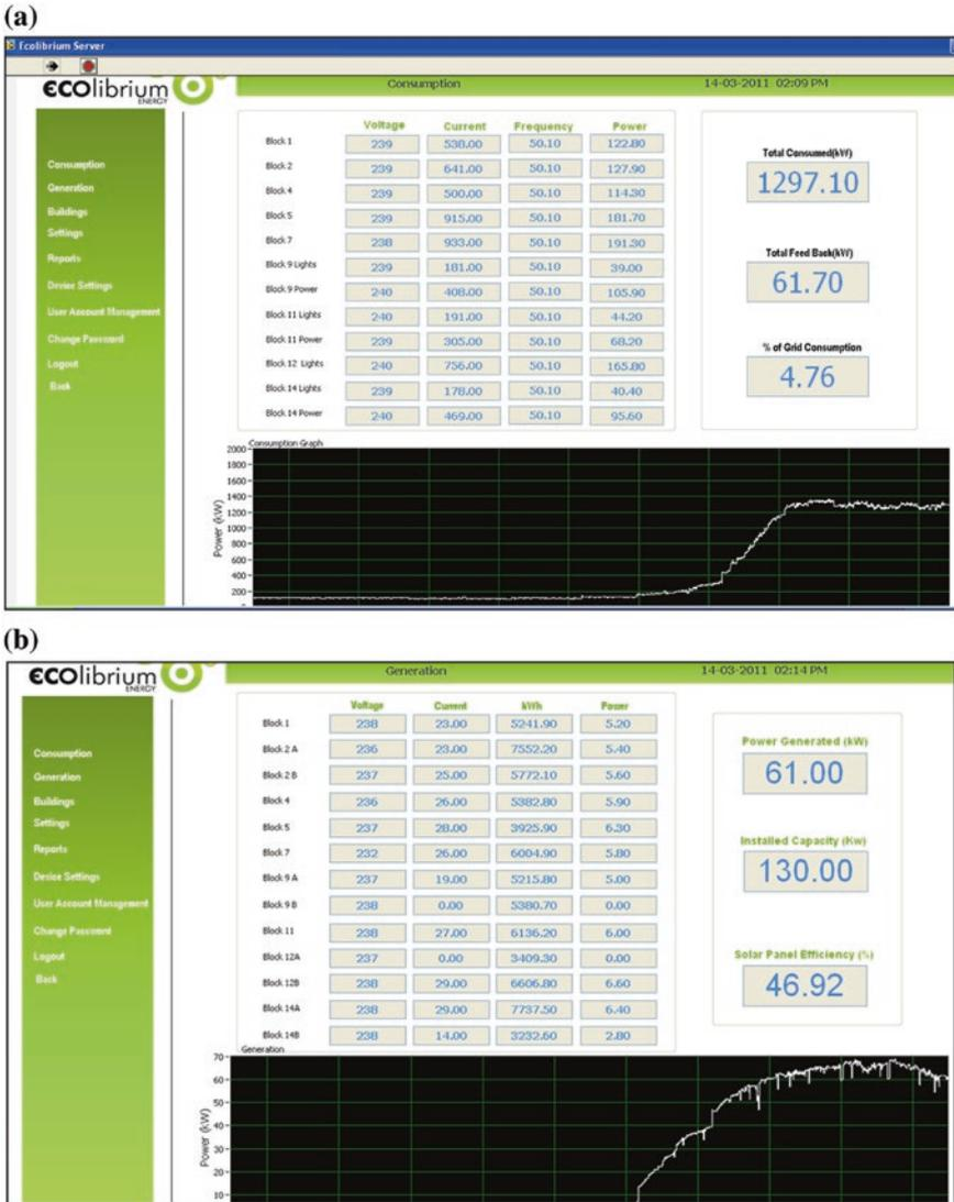
Fig. 17 a Consumption of all buildings GUI and b generation of all buildings GUI [7]
