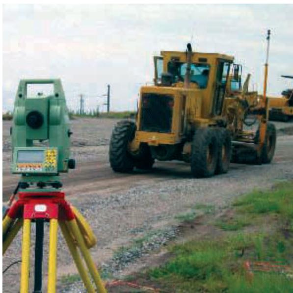
**FIGURE 2.4** Laser-guided earthmover (photo courtesy Leica Geosystems, <http://www.leica-geosystems.com>).
