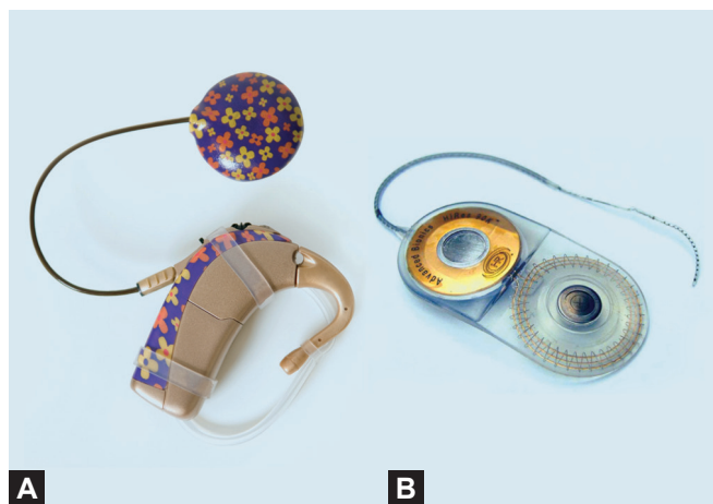
Figs. 22.2A and B: Components of a modern cochlear implant. (A) External sound processor; (B) Internal receiver stimulator.
