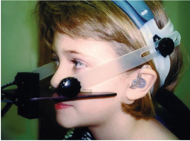
Fig. 88.3: This shows the nasometer headset in place. The nasometer collects acoustic data from the oral and nasal cavities during speech. From Kummer. 18 Reprinted with permission.
