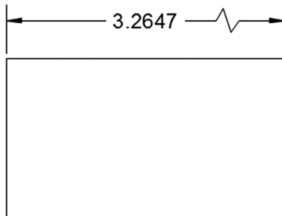
FIGURE 6.27 Jogged linear dimension.
