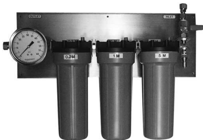
Fig. 32-5 Filter bank station. This newer filtration system steps the drinking water through a series of filters (5 micron→1 micron→0.2 micron) to enable removal of particulates, protozoa, and bacteria from the drinking water.
