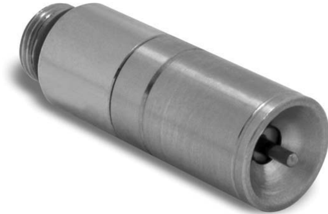
Fig. 32-10 A rodent drinking valve that is shielded to prevent bedding from entering the valve, and guarded to prevent the valve stem from being accidentally deflected.
