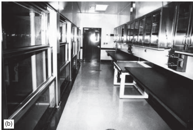
Fig. 19-14 (a) Procedure laboratories and animal husbandry suite. (b) Double-sided cubicles procedures laboratory. There are four 7' \times 4' cubicles (left), wall-mounted upper cabinets, lower work counter with vibration-free table, and two stainless-steel utility (moisture-resistant electrical outlets, air, vacuum, carbon dioxide and natural gas) service chases, all on the right-hand side. A sink is located adjacent to the door. Each cubicle has a second vertical sliding door on the opposite side (see Figure 19-14(c)) to accommodate animal husbandry service activities. (c) Double-sided cubicles animal husbandry space. There are eight 7' \times 4' cubicles (four on each side) and an animal transfer workstation against the back wall.
