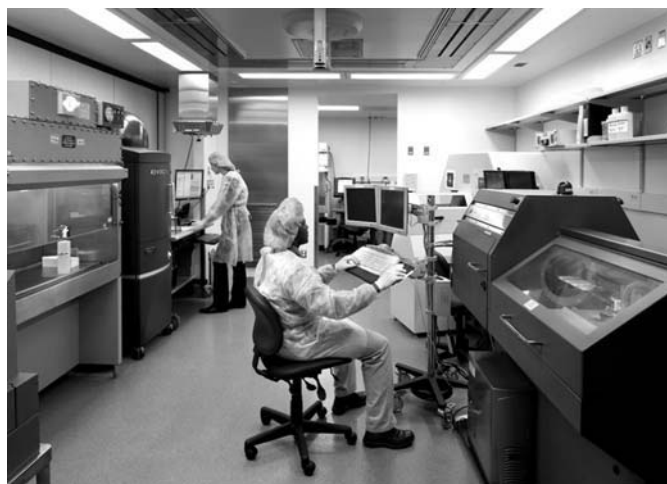
Fig. 20-7 A rodent-imaging laboratory containing various types of imaging equipment and support equipment. A combination SPECT and CT scanner is present in the right foreground, a microCT scanner is in partial view, a biological safety cabinet is located in the left foreground, and an optical imaging system can be seen in the left background.
