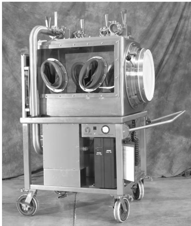
Fig. 25-8 Animal transport isolator. Photograph courtesy of Germfree Laboratories, Inc.
