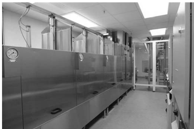
Fig. 31-15 Indexing tunnel washer. Note retracting panels above machine to create closed sections of tunnel washer.
