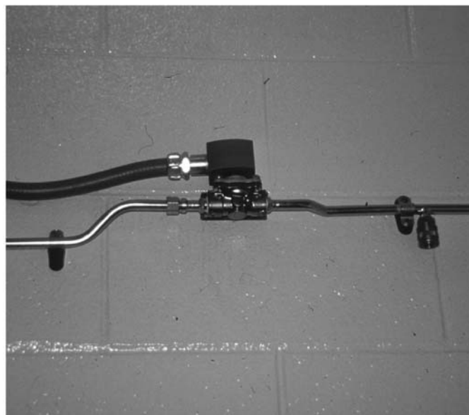
Fig. 32-11 Solenoid valve on a non-recirculating system. Electronic activation of this valve enables higher-pressure water to flush through the system to reduce biofilm development.
