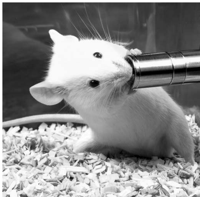
Fig. 32-4 A mouse activating the specialized drinking valve; the mouse deflects the valve stem with its mouth, enabling drinking water to pass around the O-ring and diaphragm that provide the seal.
