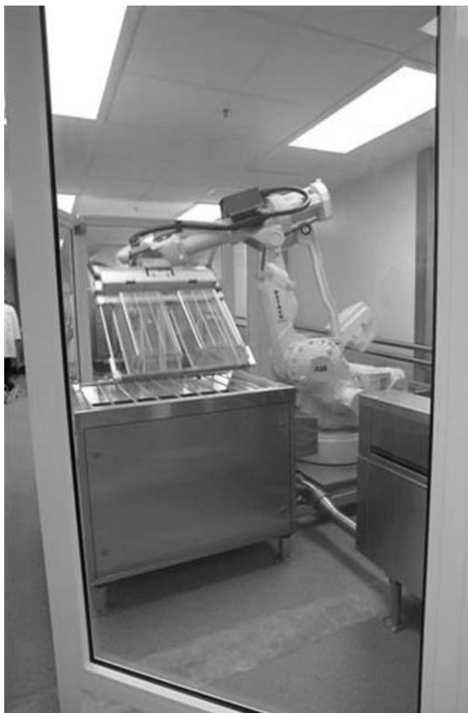
Fig. 31-14 Robotic cage cleaning. Dirty-side robot emptying soiled rodent shoebox caging.
