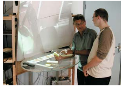
FIG. 05 TRI Setup in use in a design context: large wall projection shows collages, physical models can be enhanced with projected textures and interfaces on the table projection.
