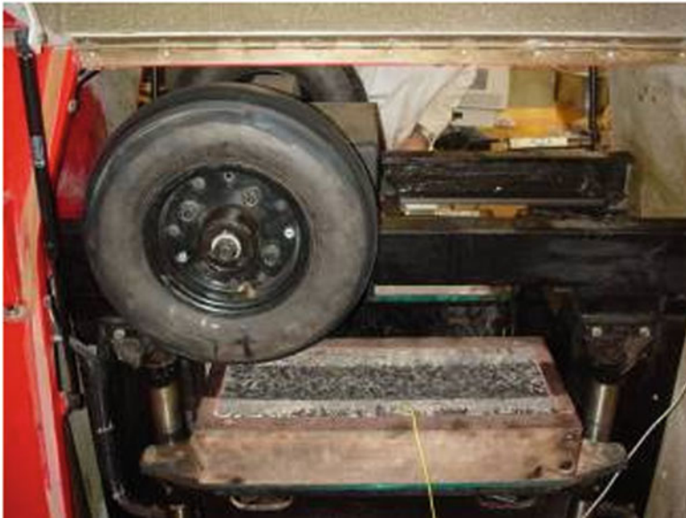
Fig. 4.21 The French Wheel Tracking Tester (FWTT)
