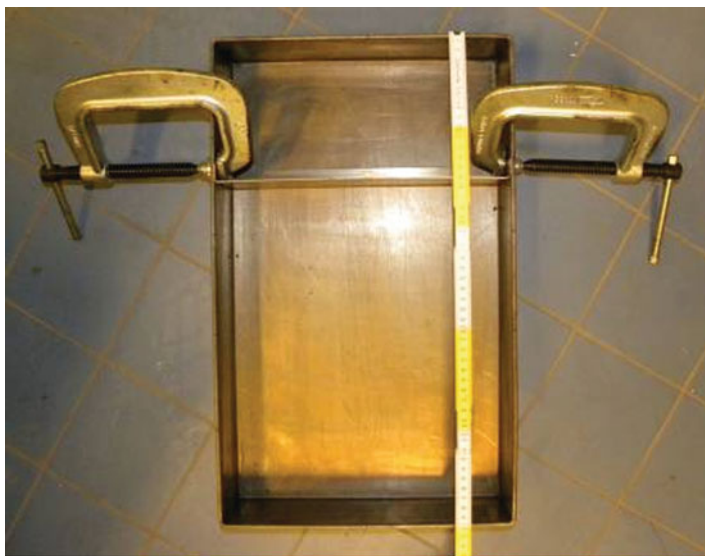
Fig. 7.2 Metal box with an internal moveable flank (TU Delft)
