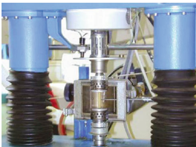
Fig. 2.30 Metravib apparatus for rheological tests of asphalt binder in LCPC
