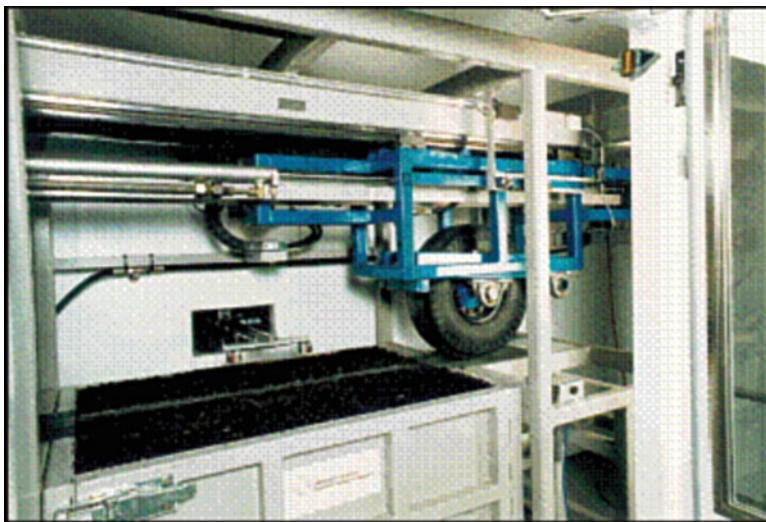
Fig. 4.33 The pavement test facility at University of Oulu in Finland
