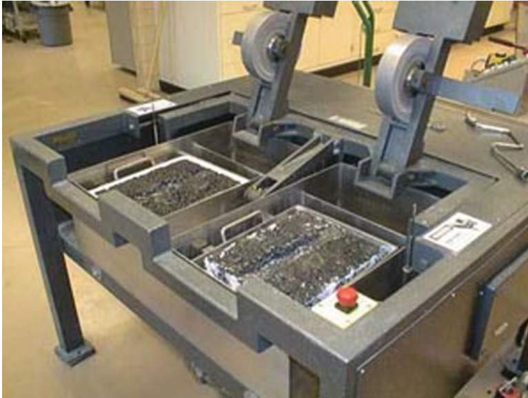
Fig. 4.25 The Hamburg Wheel Tracking Device (HWTd)
