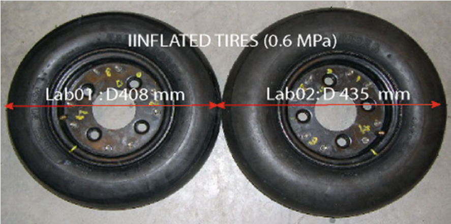
Fig. 4.70 Tyres size comparison between Lab 1 and Lab 2
