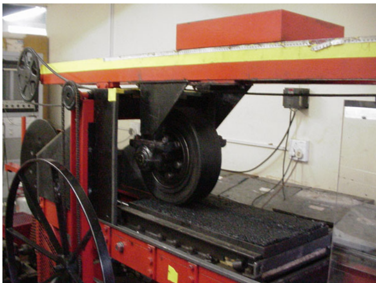
Fig. 4.31 The Transportek Wheel Tracking Tester (TWTT)
