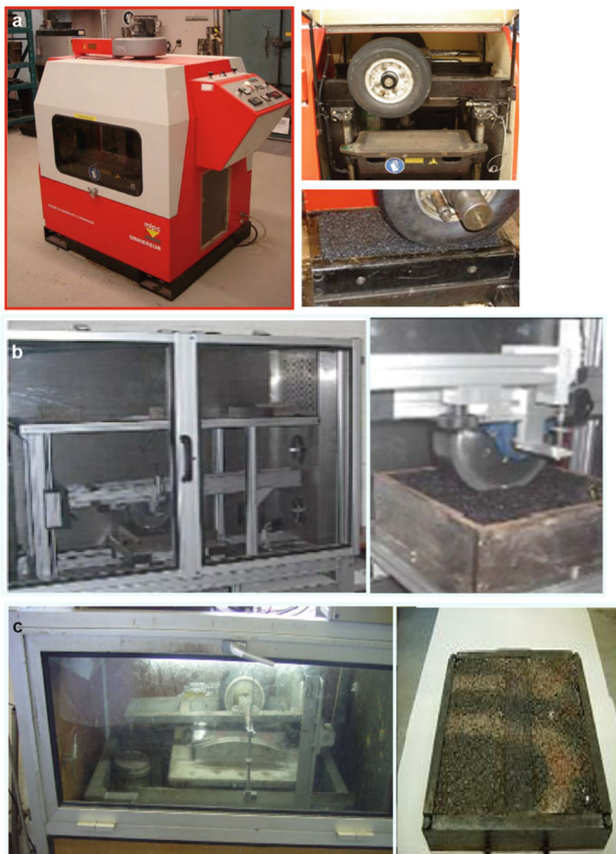
Fig. 4.39 Pictures of the three WTT devices used in the experimental programme. (a) FWTT (large size device: EN12697-22), (b) WTT-I (Small size device: EN12697-22) and (c) WTT-II (Small size device: close to the EN12697-22)
