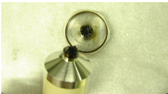
Fig. 2.75 Checking the adhesion between sample and plates after test
