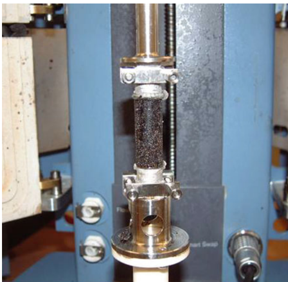
Fig. 2.38 Fatigue testing with rotational method (Bahia [7])
