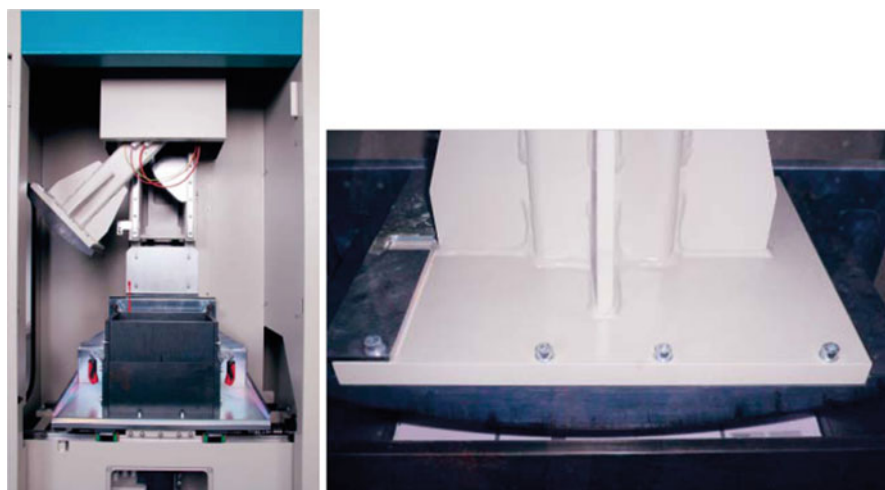
Fig. 3.5 Left: German sector compactor before use. Right: Sector compactor during use
