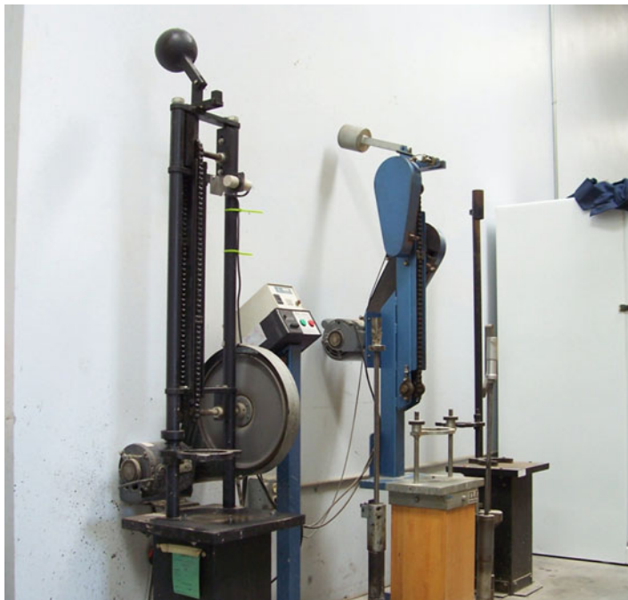
Fig. 3.1 Marshall impact hammers (Photo courtesy of PRI Asphalt Technologies, Inc.)
