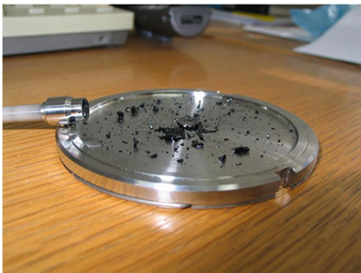
Fig. 2.64 Example of problems with fatigue test: the damage of the sample – binder F
