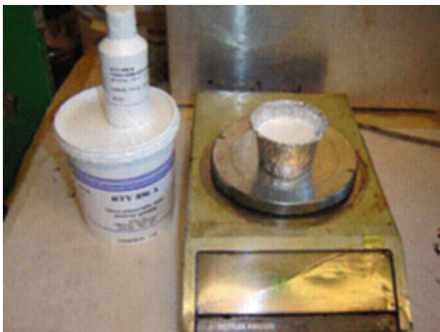
Fig. 2.71 Mixing of the pre-polymer and catalyst
