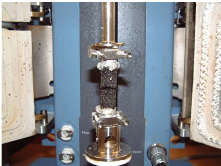
Fig. 2.39 Specimen failure after fatigue test with rotational method (Bahia [7])
