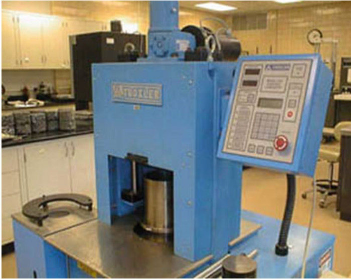
Fig. 3.6 Superpave gyratory compactor
