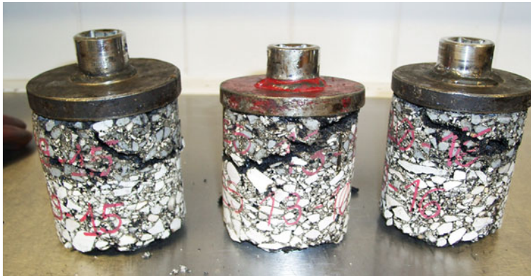
Fig. 6.21 Torque bond test: failures inside the upper layer
