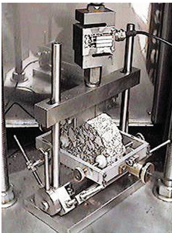
Fig. 4.7 Indirect Tensile Stiffness Modulus ( ITSM ) equipment
