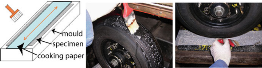
Fig. 4.54 Anti-sticking procedure. It consists of placing a sulfurized paper on the specimen and spreading a greasy soap on it and on the tyres
