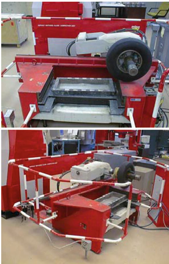
Fig. 3.3 LCPC French roller apparatus
