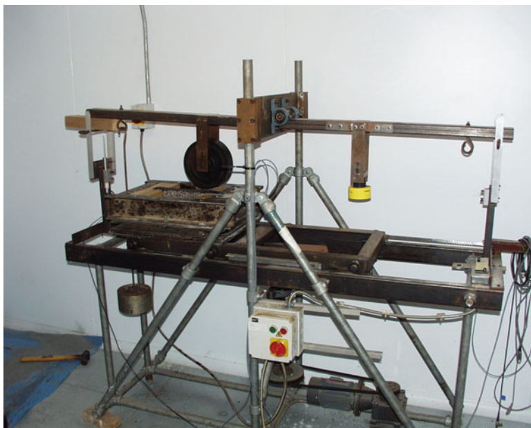
Fig. 4.24 The small-scale wheel tracking tester
