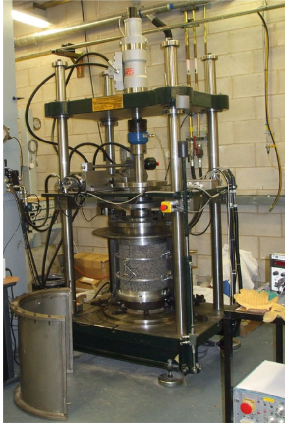
Fig. 4.20 The HCA loading frame (Tekieli [120])
