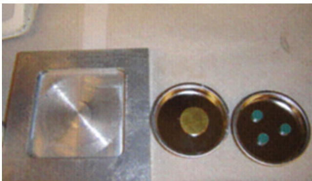
Fig. 2.72 Before making of molds, the shape for silicon rubber is needed – the metal pieces are recommended
