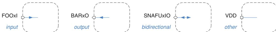
**Fig. 5.11** Terminals in schematic diagrams.
