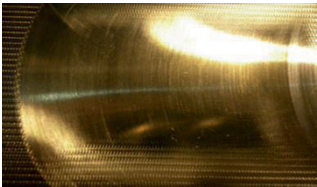
Figure 11 : Surface polished with disk 6AM Ø75, V_f = 5\text{mm/s} , N = 5000\text{rpm} , F = 30\text{N} , inclination angle = 5^\circ
