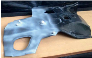
Figure 2: Tested sheet metal part partially sprayed with a white matte layer to allow acquisition with a laser scanner very sensitive to the original black colour of the part.
