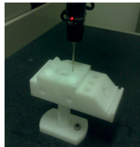
Fig. 2. CMM (Mitutoyo EURO-C544) and sample workpiece for training purposes.
