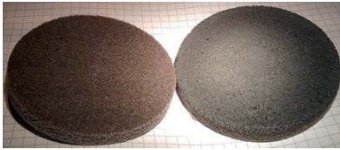
Figure 12 : New tool and fouling tool
