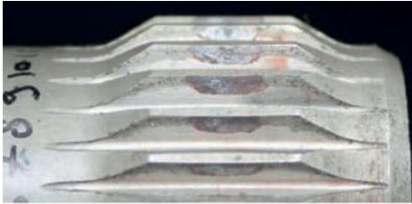
Figure 12: wear damage in crowned teeth spline couplings after test performed without lubrication.
