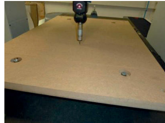
Figure 15: Measure of a Medium Density Fiberboard (MDF) free-form surface after milling with a CCM Hexagon and a continuous probe Renishaw SP25
