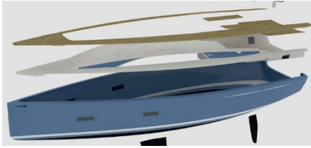
Figure 2 : The hull and deck and fiberglass structural supports.
