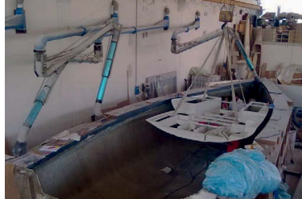
Figure 3 : The basement of the Sly 38 and the guides for transverse bulkheads.
