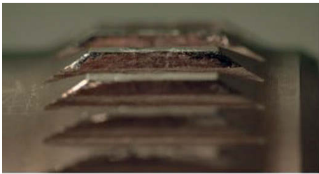
Figure 13: wear damage in straight teeth spline couplings after test performed without lubrication.
