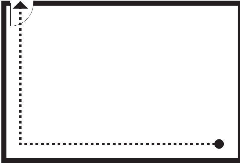
FIGURE 10.2.1-4. Acceptable travel distance path.
