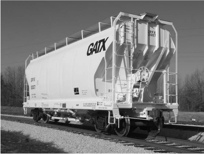
Figure 5.15 Railway car used to transport cement (courtesy of Philippe Pinsonneault, Ciment St-Laurent).
