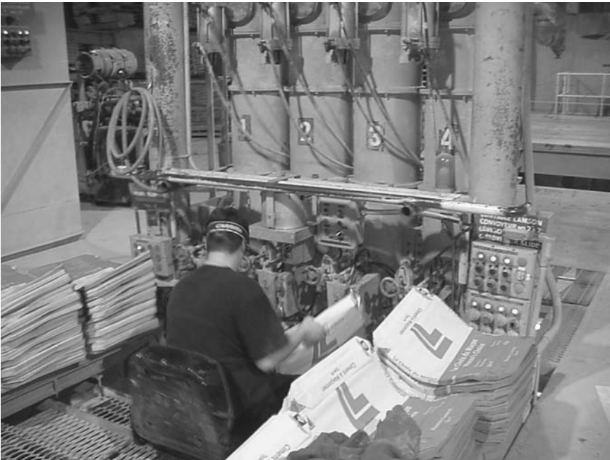
Figure 5.13 Semi-automatic bagger (courtesy of Philippe Pinsonneault, Ciment St-Laurent).
