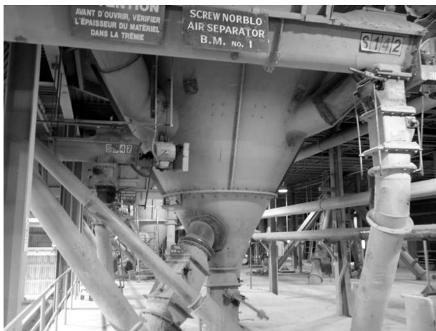
Figure 5.11b Cyclone separator (courtesy of Philippe Pinsonneault, Ciment St-Laurent).
