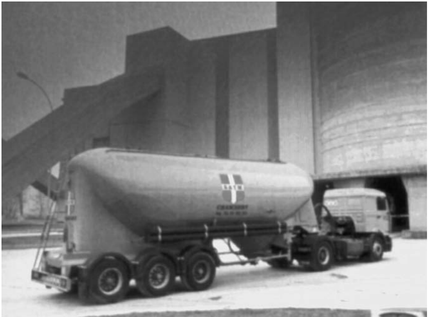
Figure 5.16 Cement tanker (courtesy of Groupe Vicat).
