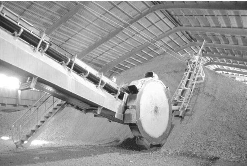
Figure 5.6(b) Reclaiming the raw materials in a pre-homogenization stock yard (courtesy of Lafarge).
