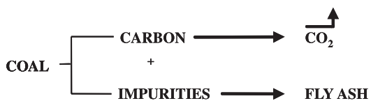
Figure 8.14 Schematic representation of the production of fly ash.
