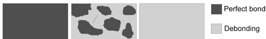
Fig. 4.1 Classification of bond into three groups: complete bond (left), uncertain bond (centre), and debonding (right)
