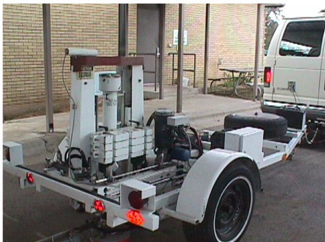
Fig. 3.1 Falling weight deflectometer (FWD)
