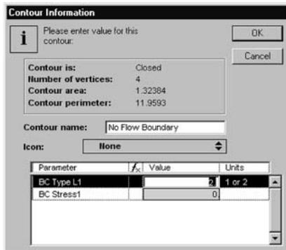
FIGURE 1.46. Contour-information dialog box used to define the type and value of the boundary-condition location defined by the portion of the domain boundary encompassed by the polytope with the black squares at each vertex.
