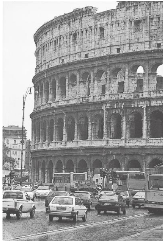
FIGURE 8.6. The Games. The Colosseum in Rome (Flavian Amphitheater) stood nearly 50 meters tall. The outside of the building consisted of three arcaded facades and an “attic” story, from which the velarium —a great canopy that shaded the spectators—was hung. A special unit of the Roman navy, whose job it was to unfurl and secure the canvas canopy, was permanently stationed here.
