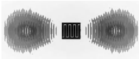
Figure 5.7 Example of the simulated GWs lobe generated by IDT
