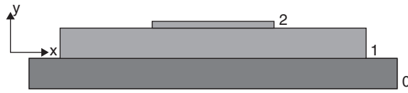
Figure 16.2 The modeled DDA block system constraining the motion of Block 2 to horizontal sliding only. Block 0 is the foundation block, Block 1 receives the dynamic input motion (horizontal – cyclic), and Block 2 responds (after Kamai and Hatzor, 2008).
