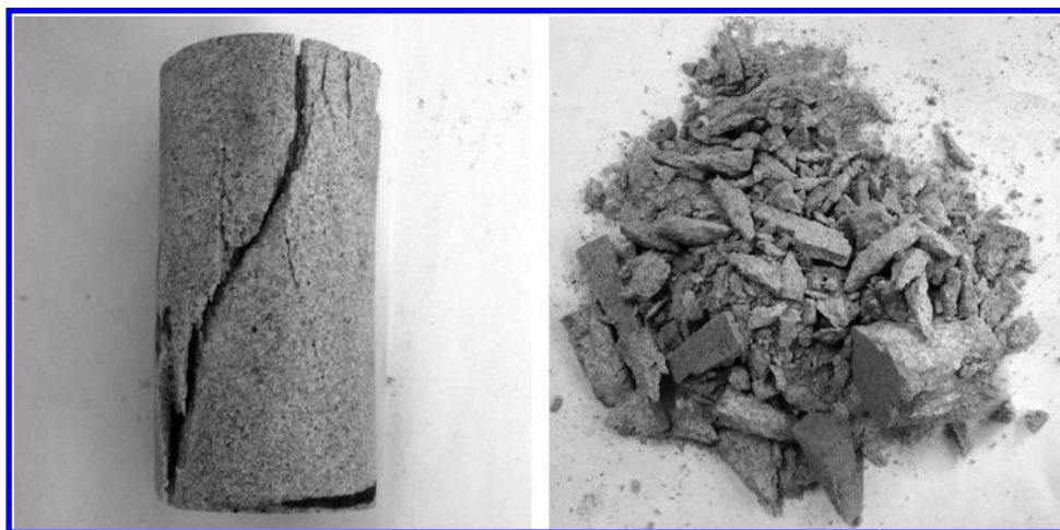
Figure 1.1 Rock specimens after failure under static (left) and dynamic (right) loads.
