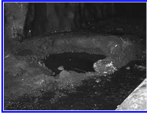
Chamber with craters after detonation (Test #3)
