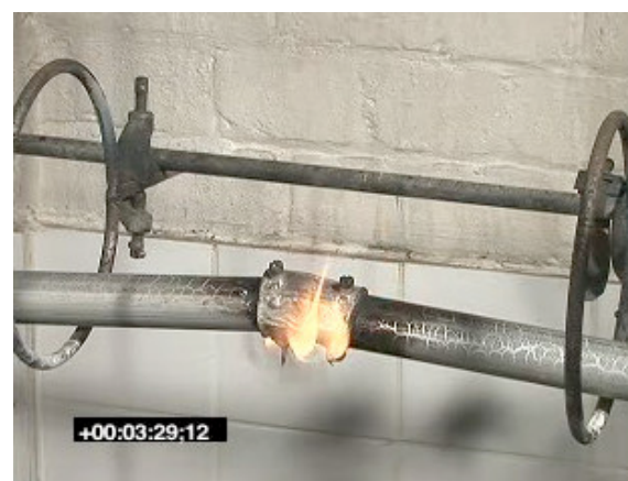
Figure 12 – Flames have increased and coupling now appears to be misshaped.
