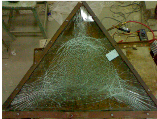
Figure 10. Failure of the Specimen # 1
