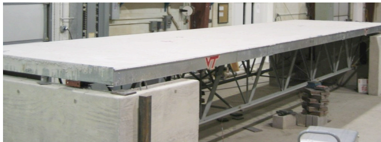
Figure 1 Single Span Floor (7 ft x 30 ft)
