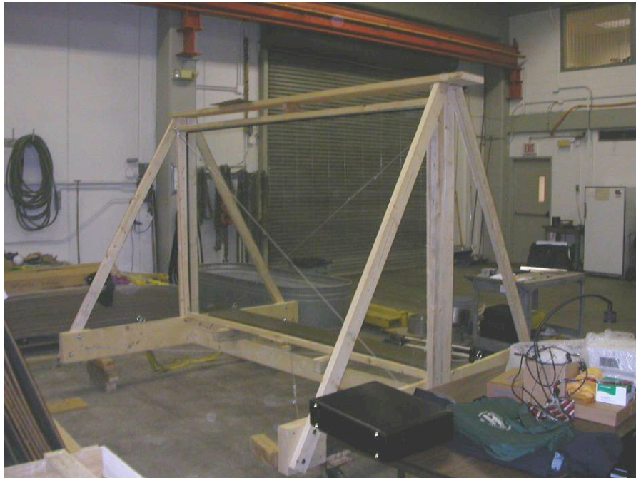
Figure 5 - Vision lite placed in wood frame for further inspection and analysis.
