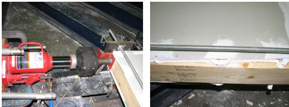
Figure 7. Condition of drywall near the loading jack and at end studs
