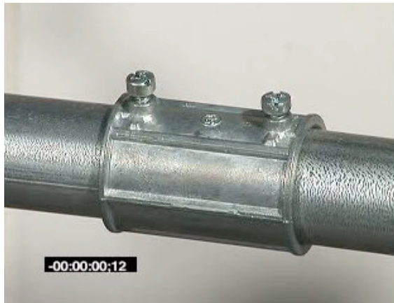
Figure 9 – Die-Cast Coupling attached to two 18" lengths of metal conduit (Start of Test).
