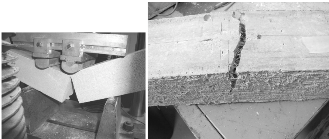
Figure 3: ASTM C1018 Specimens after failure: Plain mortar specimen (left), PVA- FRM specimen (right)
