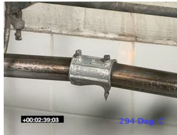
Figure 11 – Flames from the non-plenum cable are visible.
