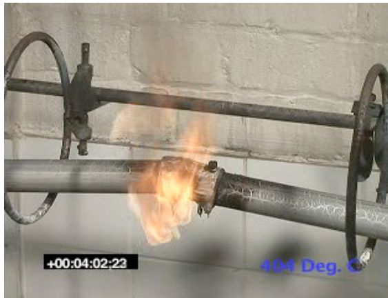
Figure 13 - EMT joint failure occurs at 404°C.
