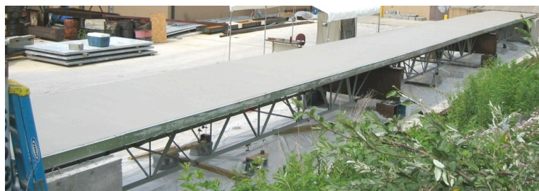
Figure 2 Three Span Floor (7 ft x 90 ft)
