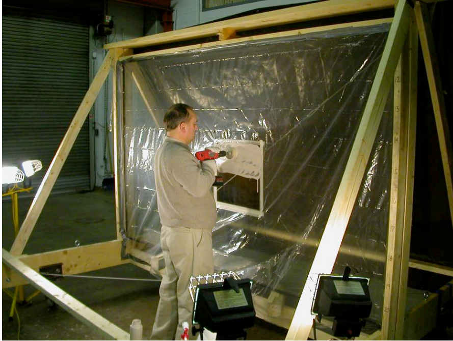
Figure 6 - View of trial cleaning with cerium oxide slurry
