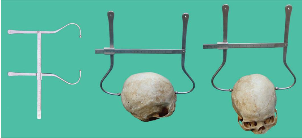
**Fig. 27.1** A head spanner and its usage for the measurement of the length and the breadth of a skull
