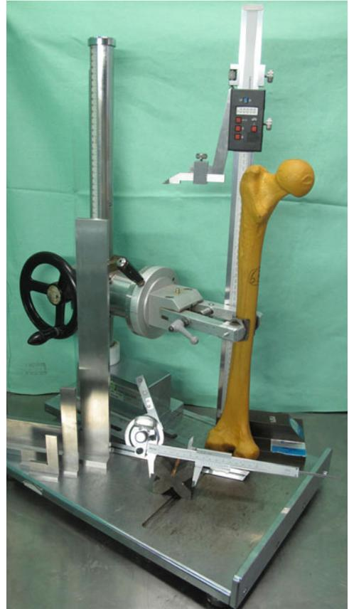
**Fig. 184.3** Three-dimensional digitizer. Points on the bone surface can be acquired with a 3D digitizer with an accuracy of microns. In this instance, a tibia, prepared with proximal and distal pots and strain gauges is being digitized (Mod. Gage-Plus-V1.5, Faro-Europe, Stuttgart-Weilimdorf, Germany, in this instance). This can assist in accurately measuring planes and measuring spatial coordinates
