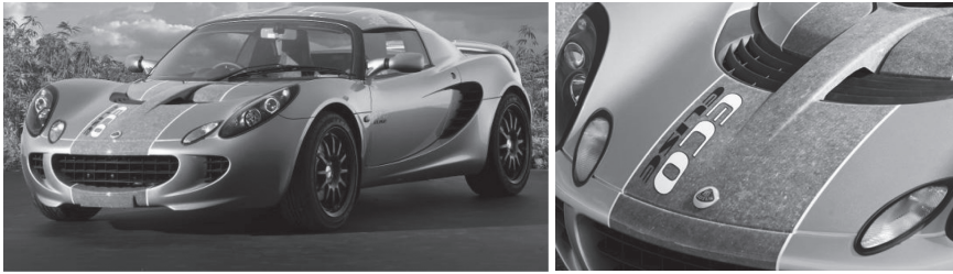
3.6 Lotus Eco Elise car and a close-up of the Eco Elise hood showing the hemp fibre pattern in the clear-finished stripe. Photos used with kind permission of Lotus, UK.
