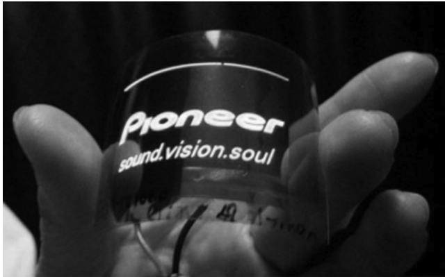
19.10 Luminescence of an organic light-emitting diode deposited onto a flexible, low-CTE and optically transparent wood–cellulose nanocomposite (from [121]).
