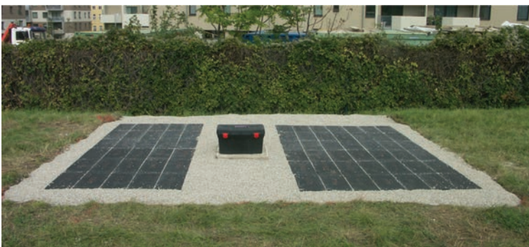
Figure 3. Photo of the test field with winter maintenance section (left), electric cabinet (center) and section without winter maintenance (right).
