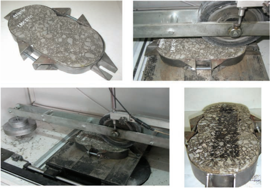
Figure 9. WTT with cores taken from the pavement.
