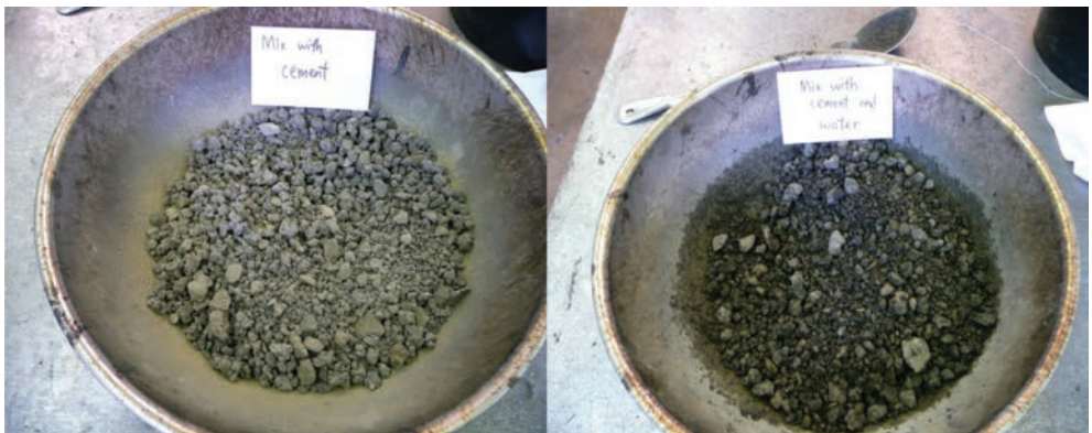
Figure 5. A sample mix after blending with cement and water.
