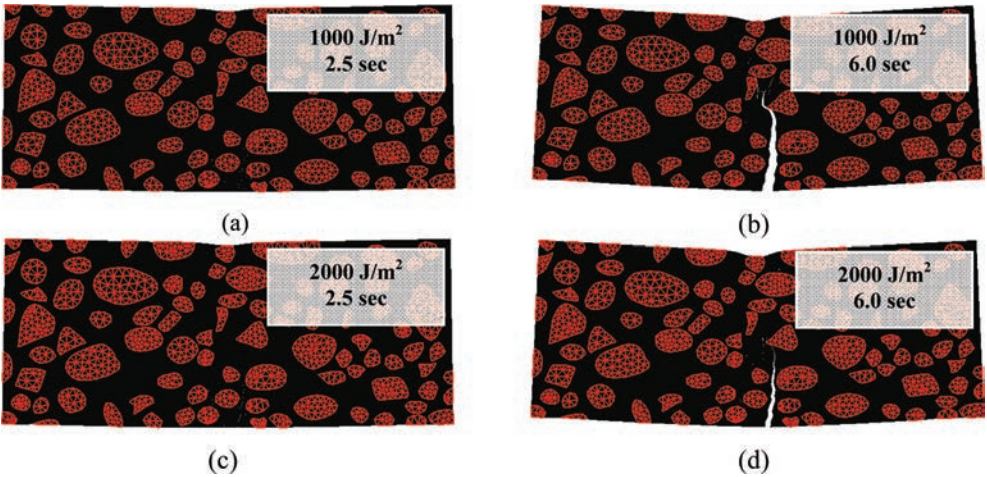
Figure 7. Progressive microstructural fracture at two simulation times, i.e. , 2.5 and 6.0 seconds, for two different G_c^{ref} : (a) and (b) 1000 J/m 2 ; (c) and (d) 2000 J/m 2 .
