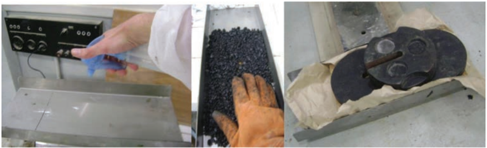
Figure 2. Asphalt Slide Test: applying ARA (left), asphalt spread on the plate (centre), load of 2,5 kPa distributed on top of the asphalt (right).
