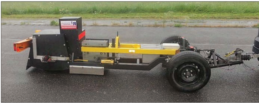
Figure 2. The tire/road Rolling Resistance measurement TUG trailer.
