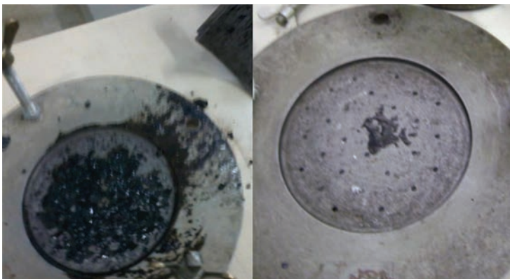
Figure 5. Compressor compacted IT loading samples showing leaching of bitumen with 5 mL ARA applied after compaction (left) and 2 mL ARA applied before compaction (right).
