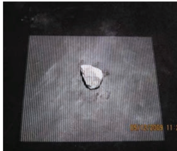
Figure 4. Projection grating on aggregates surface.
