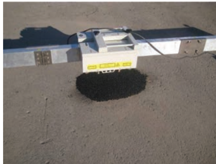
Photo 2. Measurement road surface profile condition.
