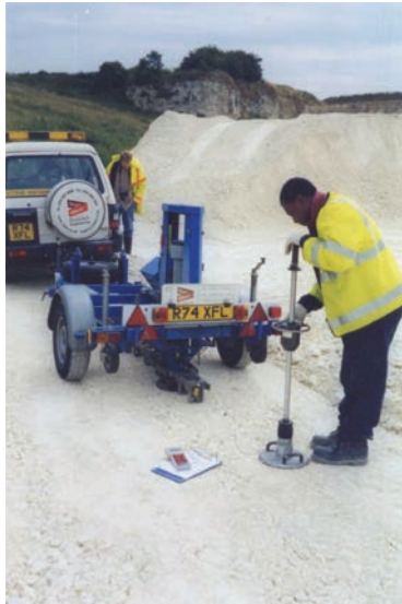
Figure 2. Falling Weight Deflectometer (FWD) and Light Weight Deflectometer (LWD) tests on a trial foundation.
