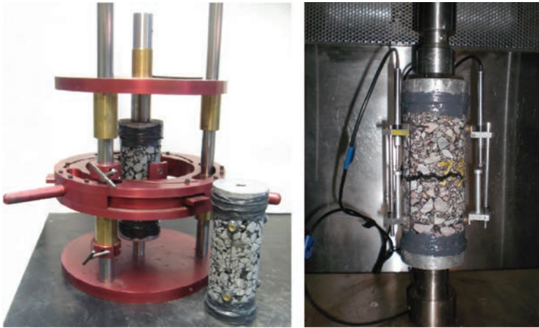
Figure 2. Specimen gluing jig and test setup with failed specimen.
