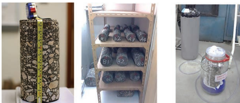
Figure 2. Photos of samples cores used in this study. 2a. Conditions of cores. 2b. Cores stored in the lab. 2c. Core stored in a glass jar filled with nitrogen.
