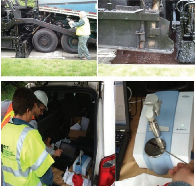
Figure 2. Sampling emulsion (top left), Novachip application (top right), ATR testing setup (bottom left), sample placement (bottom right).
