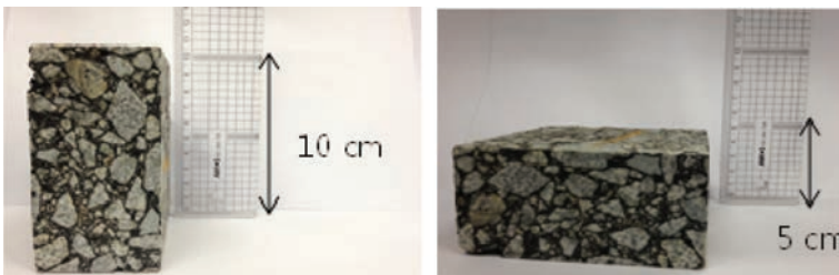
Figure 2. Direct loading test specimens.
