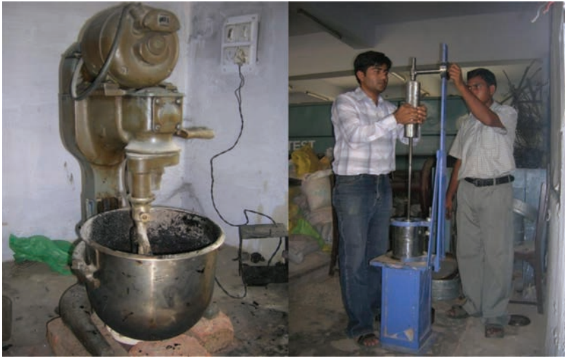
Figure 3. Mixing and compaction of DBM sample.
