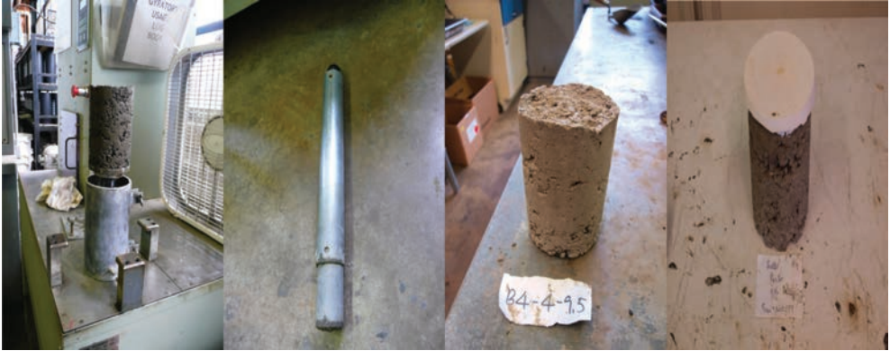
Figure 6. From left to right; proctor specimen and the steel mold, rammer for the proctor test, one day cured specimen, capped specimen after 7 day curing.
