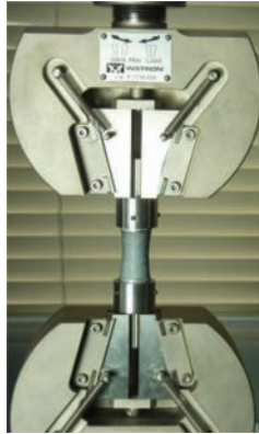
Figure 5. Details of tensile strength test set-up with mastics specimens connected to the Instron through wedge-action grips.
