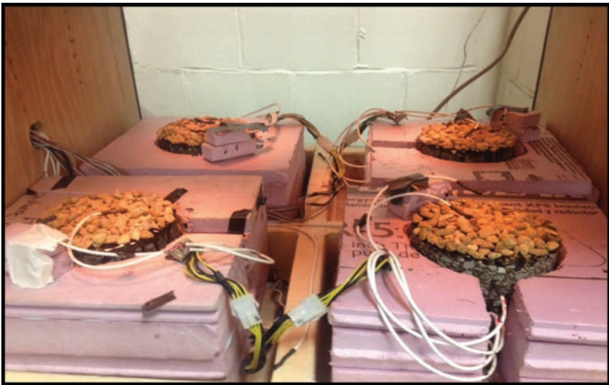
Figure 1. Four samples (with GRCS) being tested simultaneously (photo taken with side boards removed) in the solar simulator.
