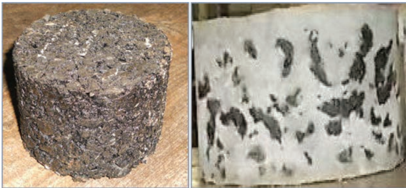
Figure 2. Cement grouted bituminous sample before and after grouting.
