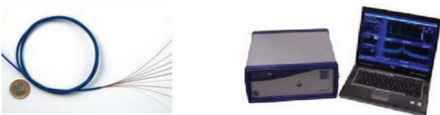
Figure 2. Fiber optic cable used as distributed sensor and measurement system.
