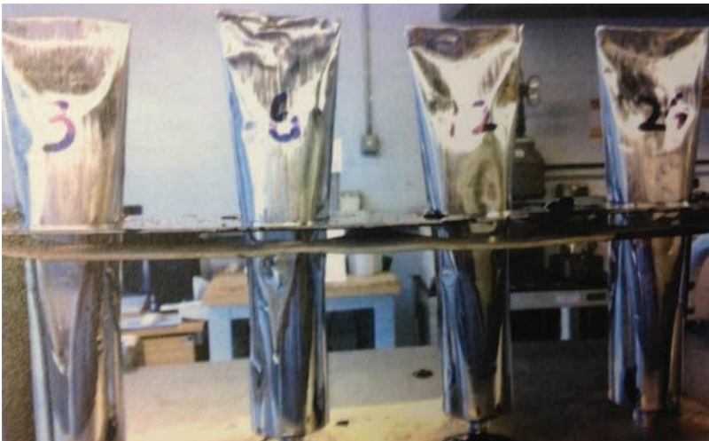
Figure 2. Toothpaste tubes in a rack prior to placing in the oven.
