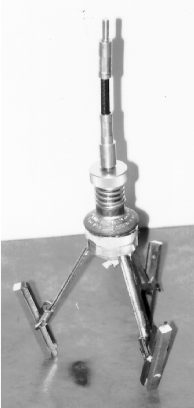
Fig. 5.12 Cylinder Hone Used for Surface Preparation of the External Pile Wall
