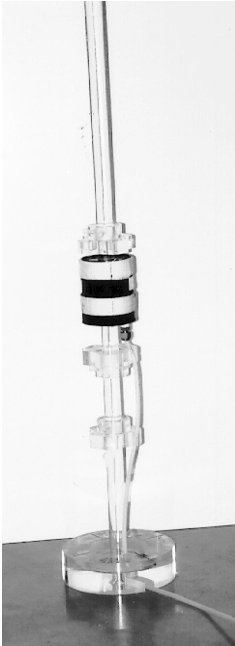
Fig. 5.13 Photograph of the Strain Gage Installer
