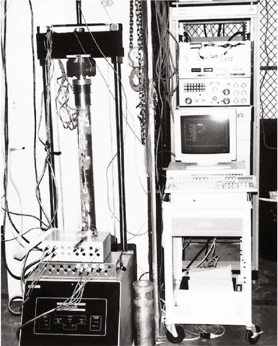
Fig. 5.26 Load Trac Loading Machine Used to Calibrate The Pile. Photograph shows (1) Computer-controlled LoadTrac machine, (2) Internal pile wall being calibrated, (3) Bridge completion boxes, and (4) MTS machine in the background.
