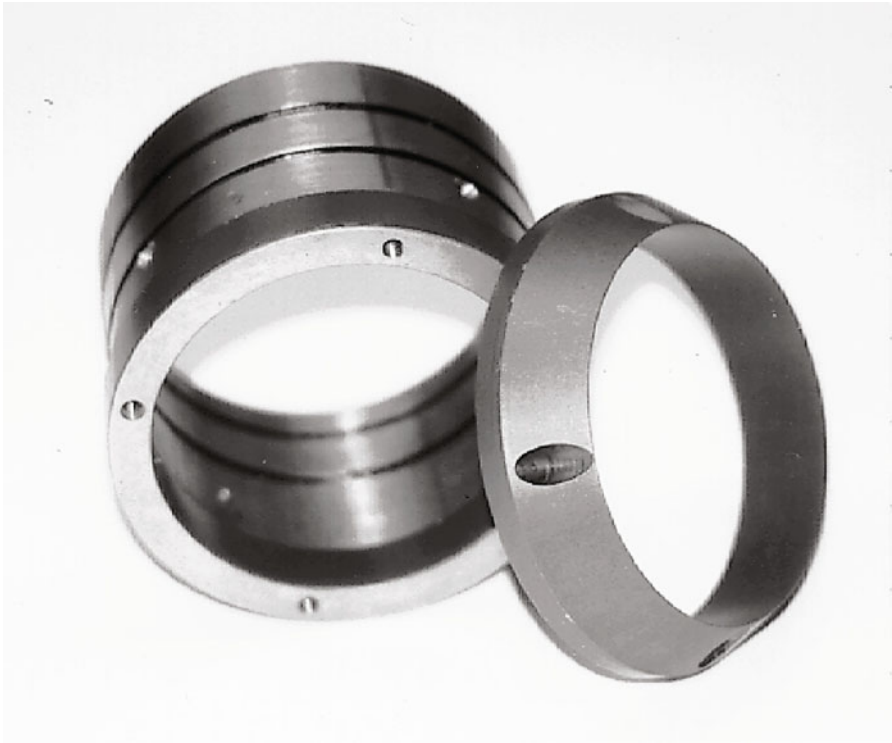
Fig. 5.8 Photograph of Pile Shoe and Cutting Shoe. Photograph shows (1) Cutting shoe (to the right), (2) Pile shoe (to the left), (3) Holes to connect cutting shoe to pile shoe, (4) Two O-ring grooves on each side of the pile shoe, and (5) Holes used to connect pile shoe to external pile wall.
