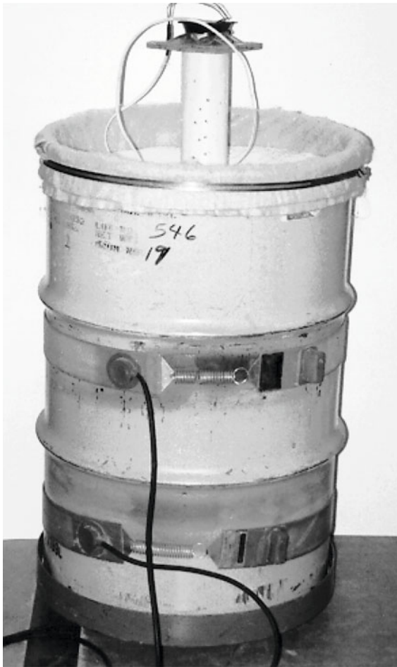
Fig. 4.17 Photograph of the Sand Drying Drum
