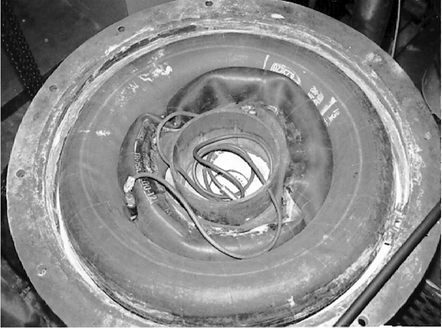
Fig. 4.5 Photograph of the Pressure Ring and Rubber Tires
