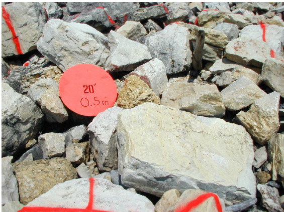
Fig. 3. Limestone riprap showing degradation caused by natural freezing-thawing (Graham et al. 2007)
