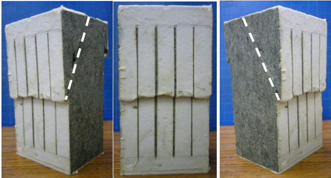
(a) undrained test under axial strain rate of 0.01%/min
