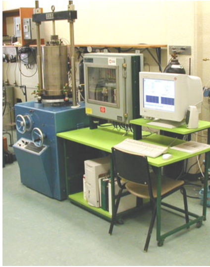
Fig. 14. High-temperature, high-pressure triaxial equipment at the University of Manitoba
