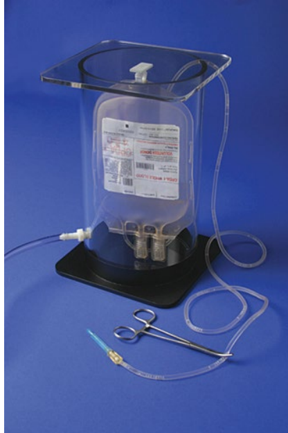
Figure 2.1 Proper set up of blood collection bag within vacuum chamber. Source: Animal Blood Resources International. Reproduced with permission.
