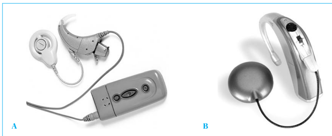
FIGURE 13-31 Photograph of the external components of two implant systems, (A) one with a body-worn processor (photo courtesy of Phonak) and (B) the other with an ear-level processor (photograph courtesy of Advanced Bionics® Corporation).
