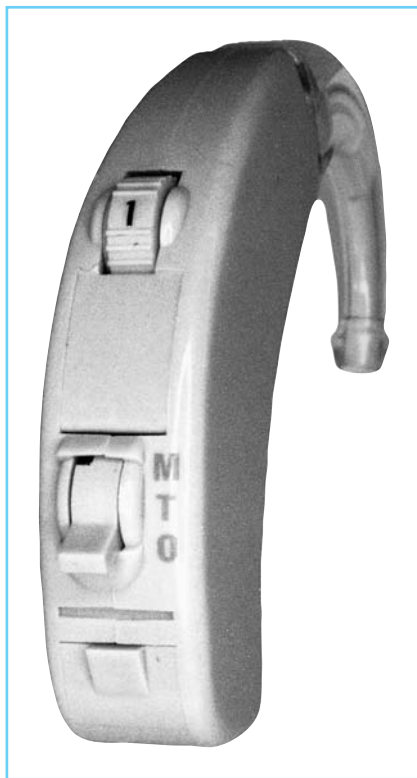
FIGURE 13-9 Photograph of a BTE hearing aid, with an MTO switch and rotating volume control. (Courtesy of Siemens Hearing Instruments, Inc., Piscataway, NJ.)
