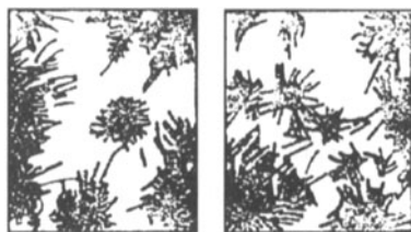
Figure 4.4 The Needle-like Crystals in Cement Paste
