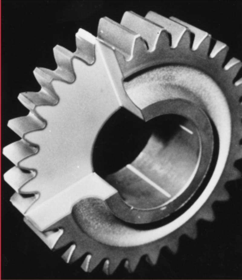
**P**hotograph of a steel gear that has been “case hardened.” The outer surface layer was selectively hardened by a high-temperature heat treatment during which carbon from the surrounding atmosphere diffused into the surface. The “case” appears as the dark outer rim of that segment of the gear that has been sectioned. Actual size. (Photograph courtesy of Surface Division Midland-Ross.)
