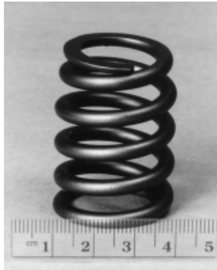
**FIGURE 20.7** Photograph of a typical automobile valve spring.
