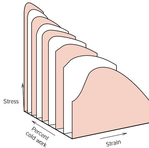
**FIGURE 8.20** The influence of cold work on the stress–strain behavior for a low-carbon steel. (From *Metals Handbook: Properties and Selection: Irons and Steels*, Vol. 1, 9th edition, B. Bardes, Editor, American Society for Metals, 1978, p. 221.)
