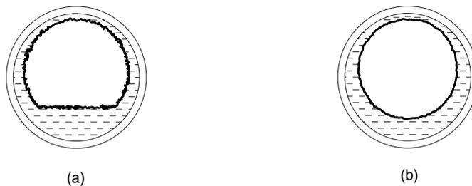
Figure 12.45. Flow patterns in condensation. (a) Stratified flow (b) Annular flow
