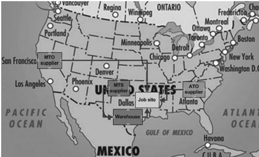
FIGURE 2.7 SC configuration: Level 1.
