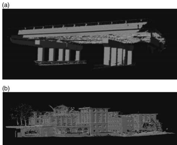
FIGURE 16.4 Example 3D models generated from laser scanned data: (a) a bridge model, (b) a building model.
