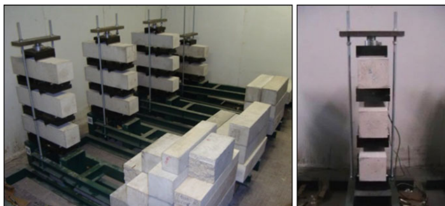
Fig. 2 General view of creep test specimens (overview -left- and column detail -right-)
