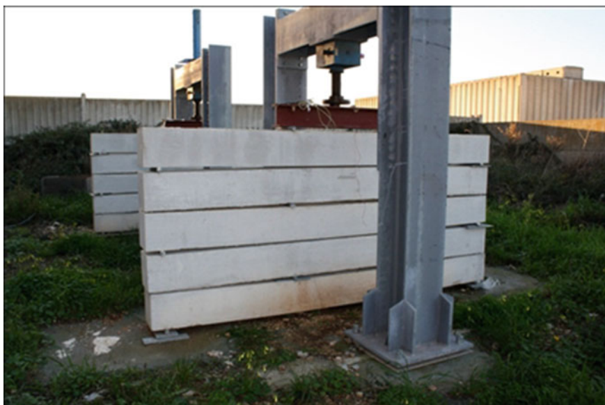
Fig. 1 The two exposure loading frames
