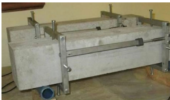
Fig. 4 Drying shrinkage test specimens [8]
