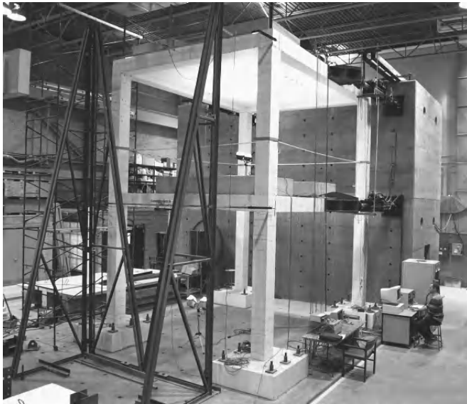
Figure 9.1. Two-storey reinforced HPC building with reaction wall
