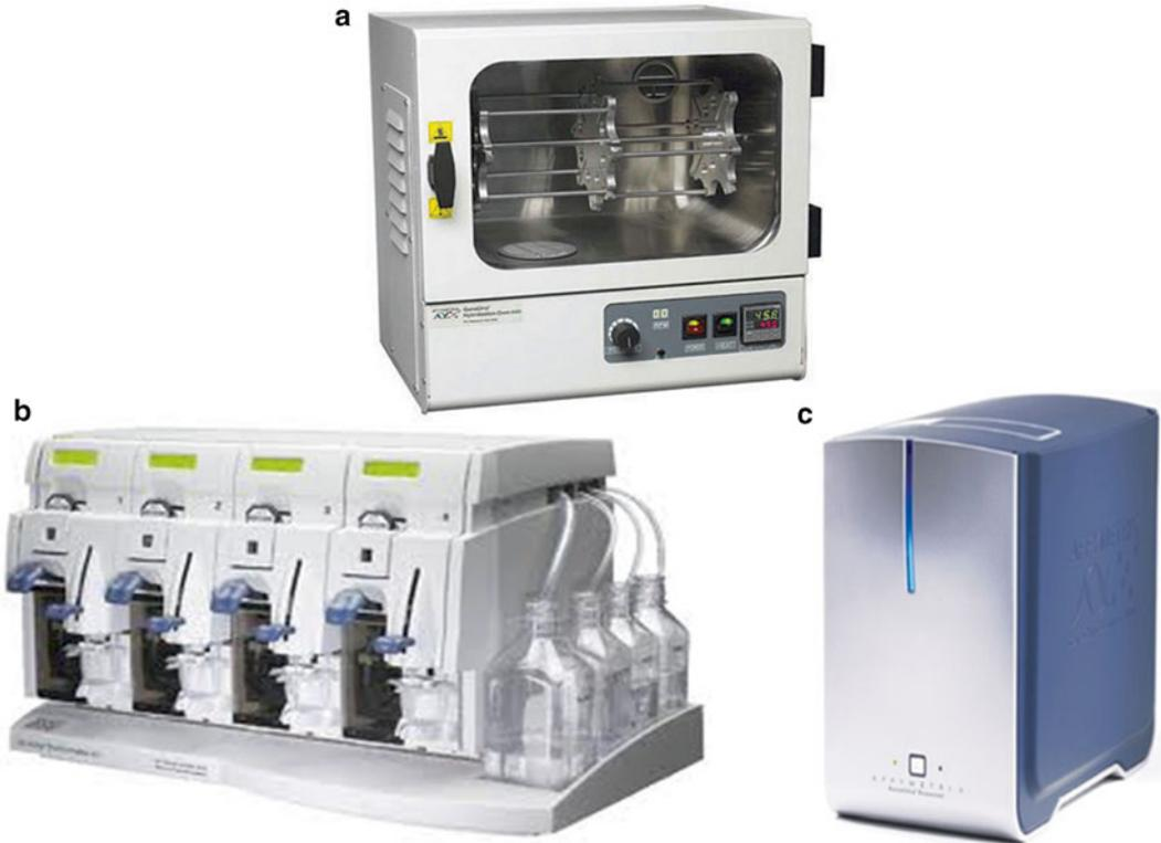
**Fig. 3** Affymetrix instruments. (a) Hybridization oven. (b) Fluidics station. (c) Scanner
