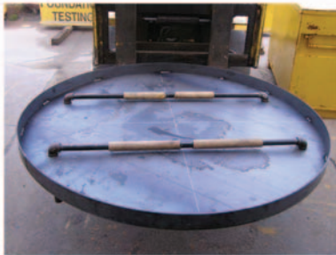
Figure 1. Tube-a-manchette underside of grout plate
