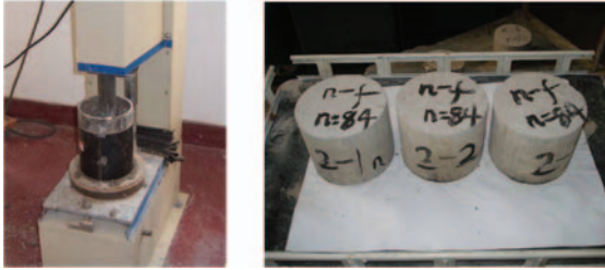
Fig. 4 Heavy compaction apparatus and specimens
