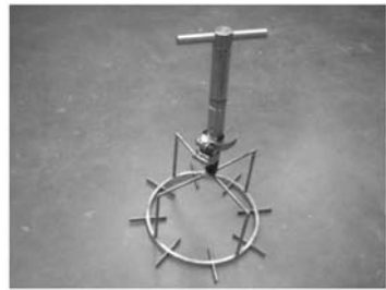
Figure 5. The new vane connected to the H-60 torque instrument.
